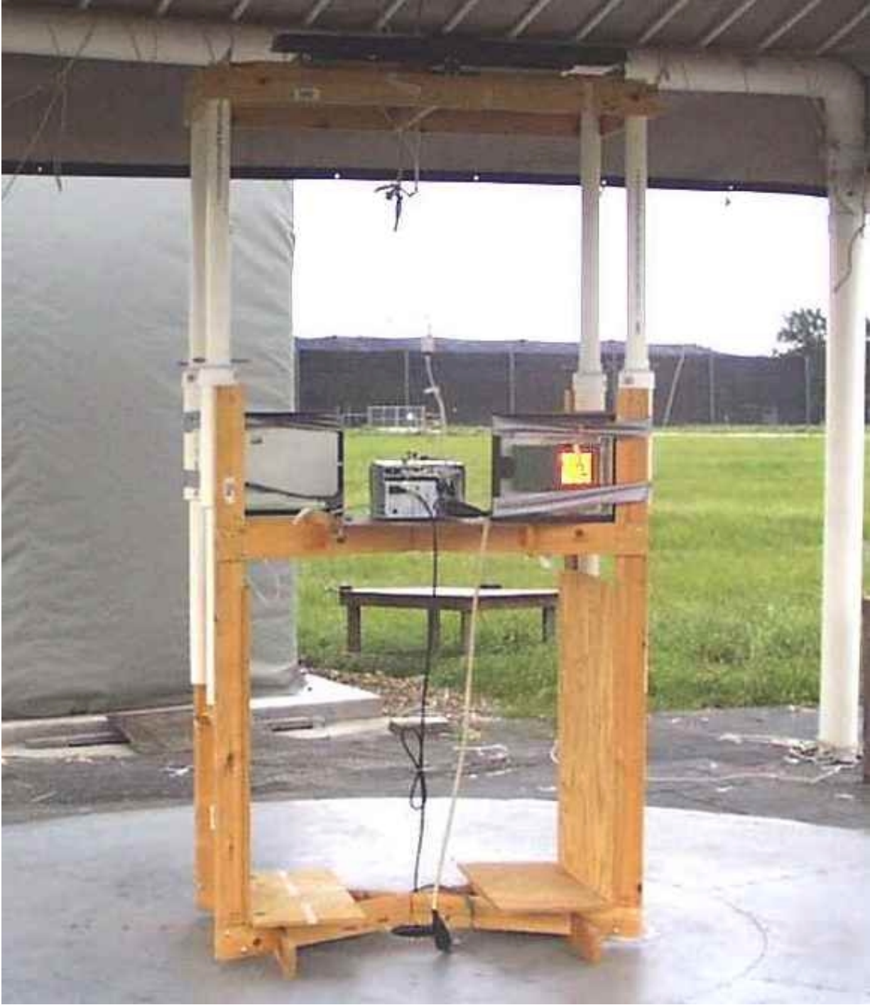
Radiated Emissions OATS Test Setup
