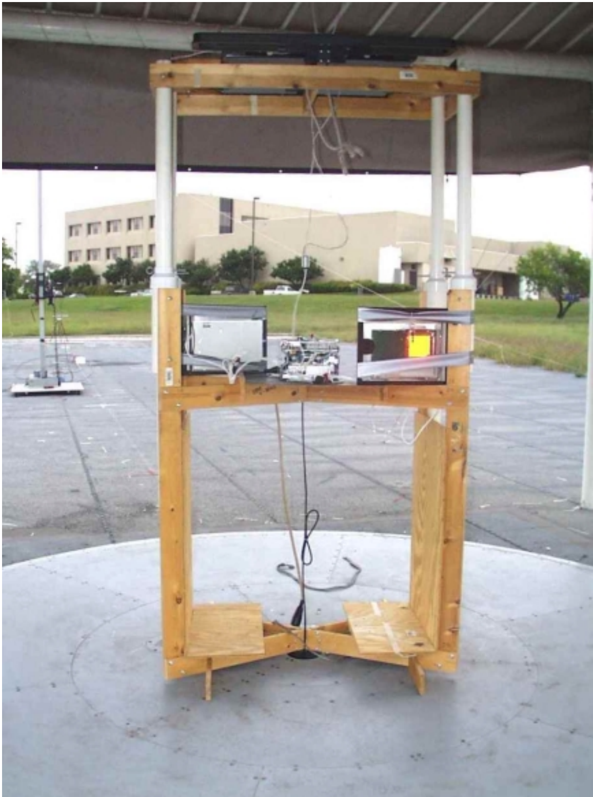
Radiated Emissions OATS Test Setup
