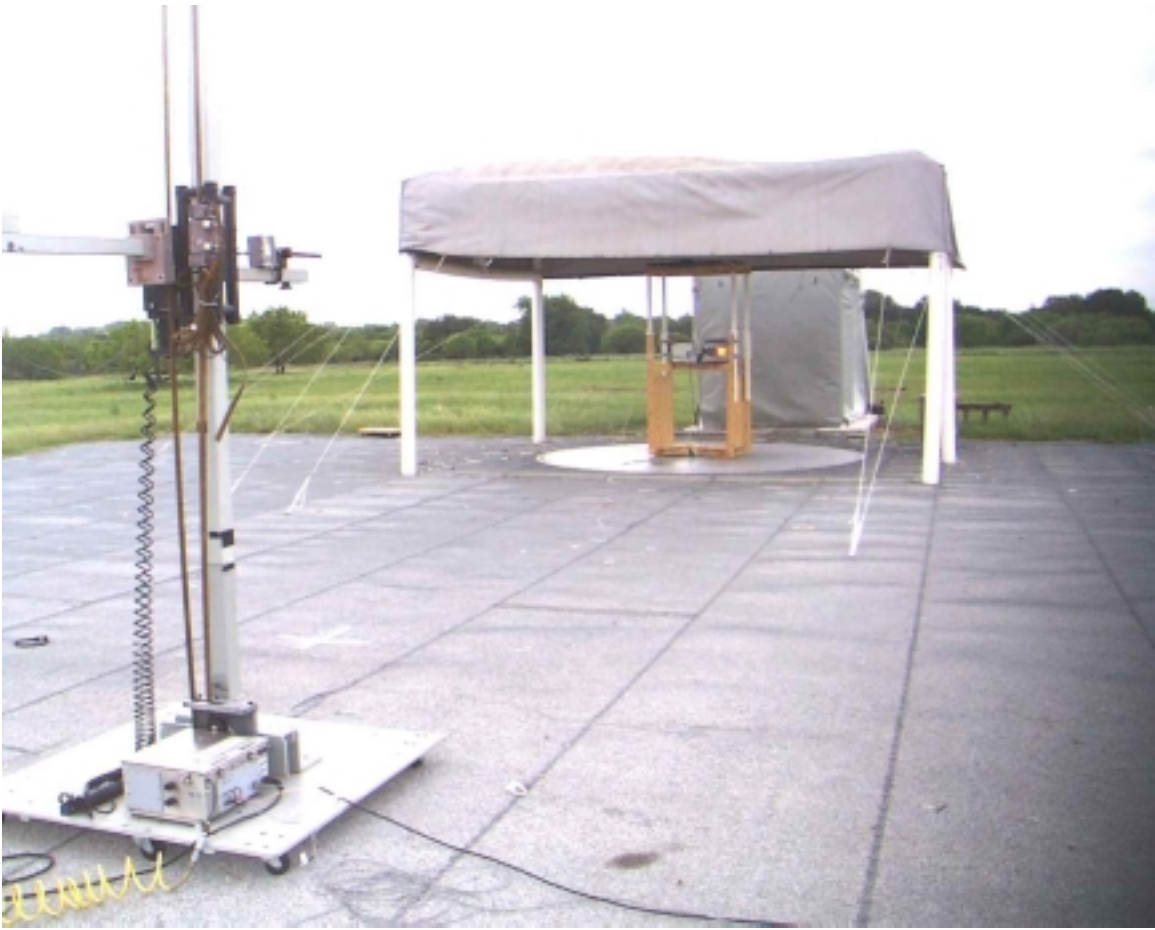
Radiated Emissions OATS Test Setup
