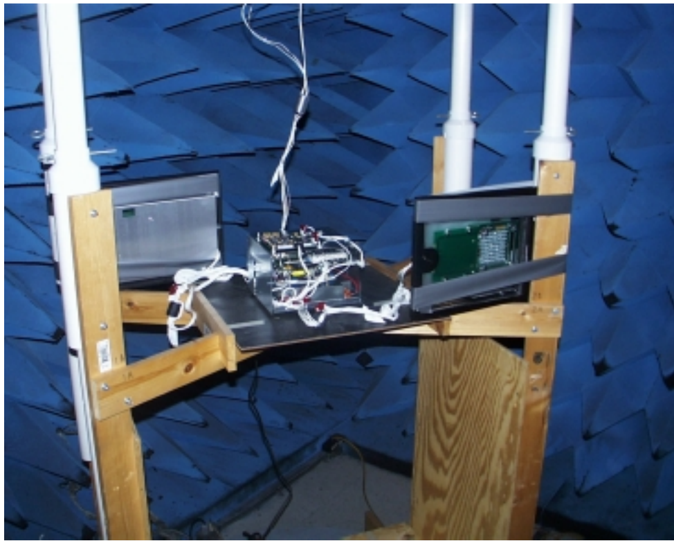
Radiated Emissions Pre-scan (Anechoic) Test Setup
