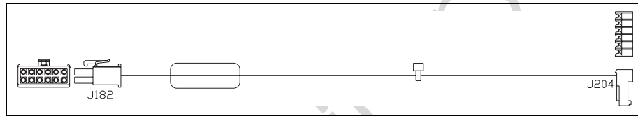
Figure 9: Light/Multi-Protocol Cable (R20773-G4)
