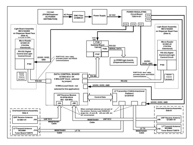
Figure 3-3: Encore Full System Block Diagram
