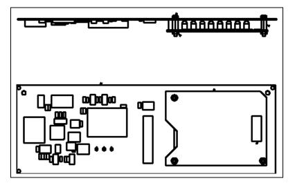
Figure 4-35: M01218A00X Light/Micro Reader PCB
