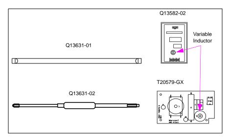
The Q13631-01 plastic flat-blade is used the same as a screwdriver. It is used with Q13582-02 and fits the slotted head of the variable inductor located on the overhead antenna PCB.
