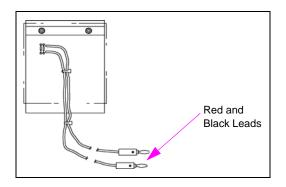
Set the multimeter to DC voltage. Connect the red and black leads of the standard multimeter to the field strength sensor board leads. As the antennas are tuned by incremental adjustments to the antenna's variable inductor (similar to a tuning pot), voltage reading increases or decreases. The field strength sensor board allows you to find the voltage peak, which is the tuning target.
