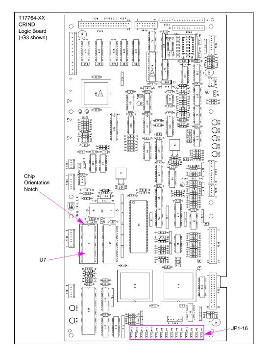
Figure 7-3: CRIND Logic Board (T17764-XX)
