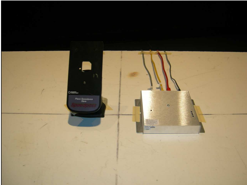
Figure 1: Radiated Emissions Test Setup – 45 Degree Angle
