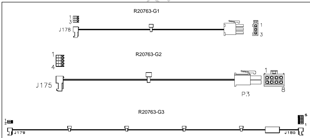
Figure 4-16: Power Supply Cables
