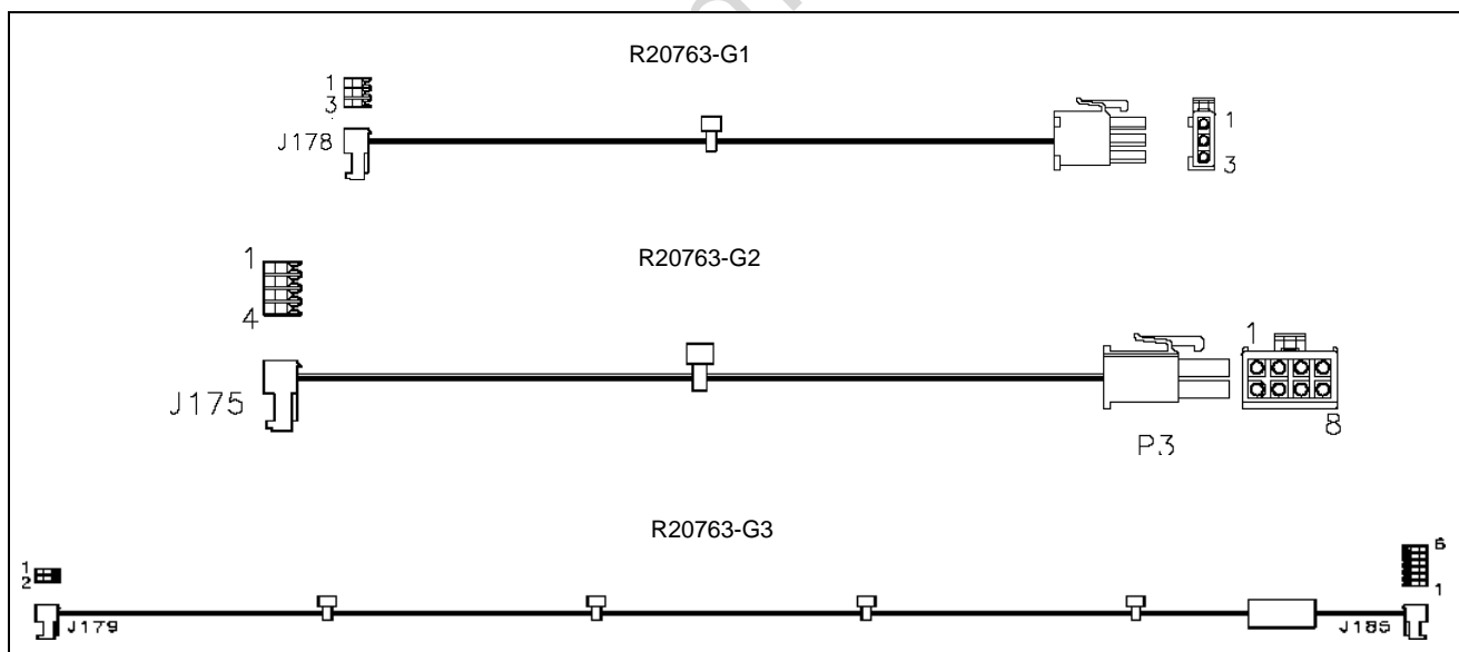
Figure 4-16: Power Supply Cables
