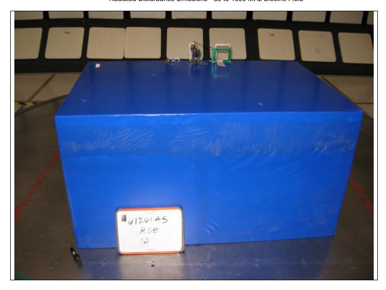
RFID Reader (EUT) in center with power/data connection board on left, antenna on right. From preliminary testing it was determined that the reader was worst in the upright position as shown.
