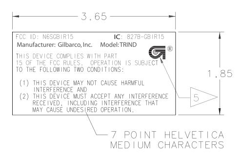
PART NUMBER N23951 10 Label 3: FCC and IC Interntional Radiator Label Units are inches. Location: interior to dispenser on sheet metal for mounting the Gateway board (T20678 G1). Page 4 of 4
