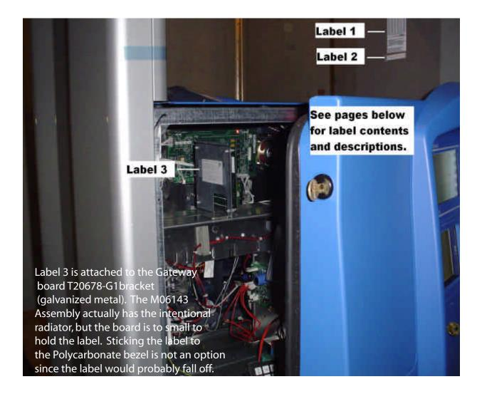
FCC and IC label locations on Encore S series fuel dispenser for N6SGBIR15 TRIND
