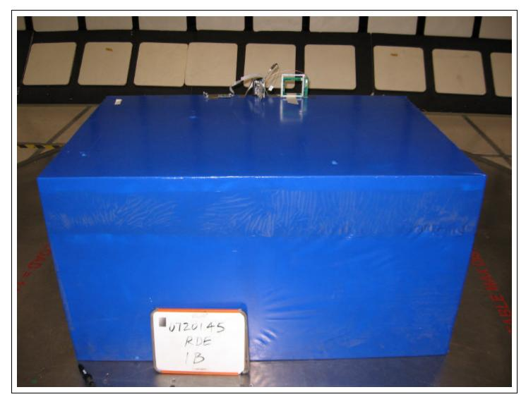
RFID Reader (EUT) in center with power/data connection board on left, antenna on right. From preliminary testing it was determined that the reader was worst in the upright position as shown.
