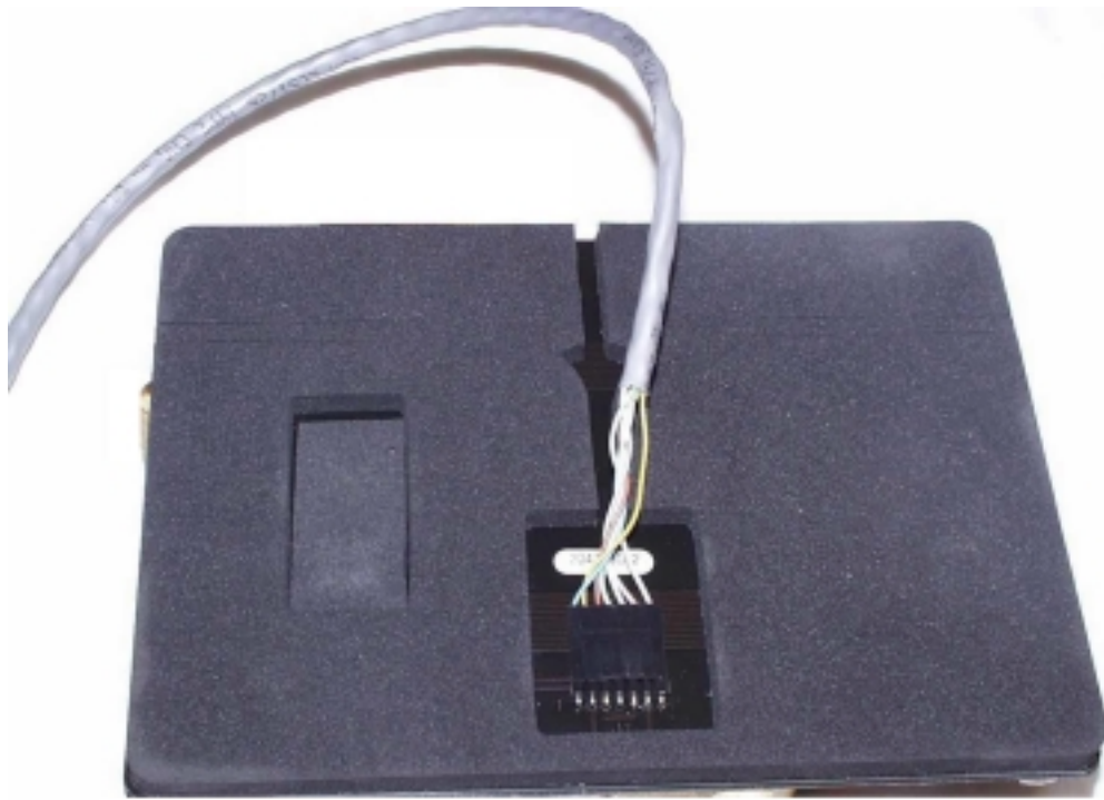
Rear View of Mat Showing Connector and Cable
