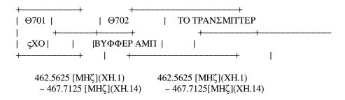
THE VCO OPERATING FREQUENCY FOR THE RECEIVER IS 440.8625 [MHz] (CH.1) TO 446.0125 [MHz] (CH.14) AS THE FIRST LOCAL OSCILLATOR, INJECTED THROUGH THE BUFFER AMP Q702 INTO THE FIRST TR MIXER Q7
