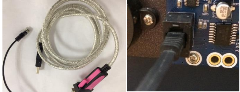
T-Cable and port of connection on CA3000L
