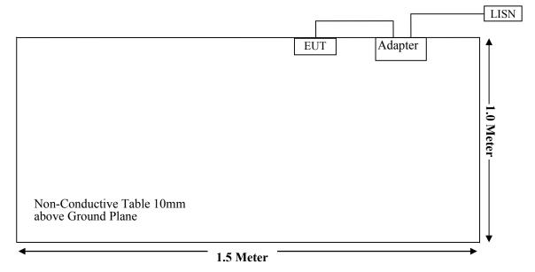
For Radiated Emissions (Below 30 MHz):
