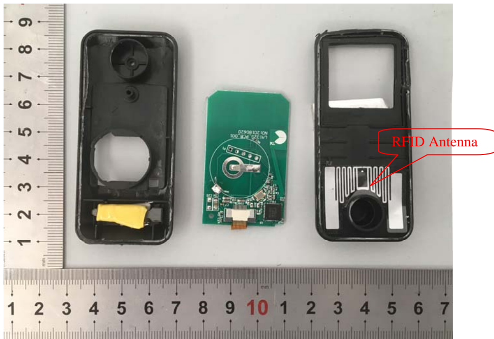
EUT – Cover off View-2
