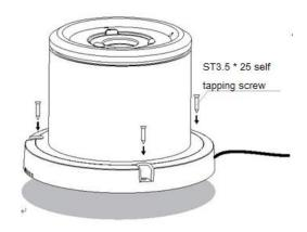
Use three self tapping screws ST3.5 \* 25 to fix the all-in-one machine on the desktop, and connect the power cable, network cable and USB cable to complete the installation (select the network cable or USB data cable according to the actual needs).
