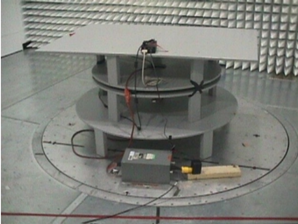
Conducted Emissions Test Configuration for Activator
