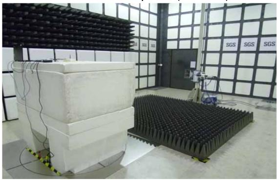
Radiated Emission Set up Photos (Front View)
