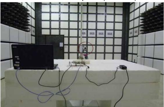
Radiated Emission Set up Photos (Below 1GHz)
