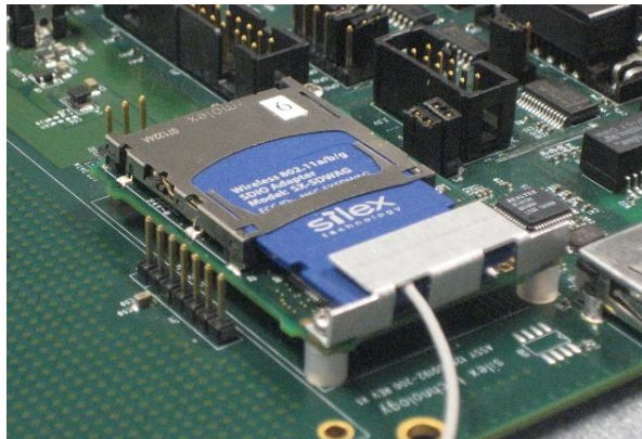
Figure 3 Securing the SX-SDWAG-02 with Optional Bracket
