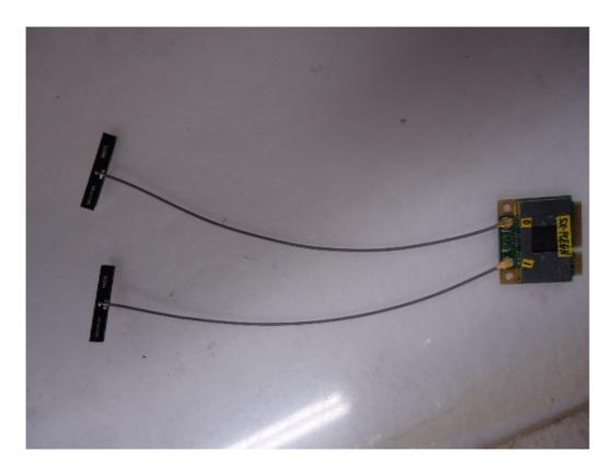
with WiFi PCB Substrate Antenna
