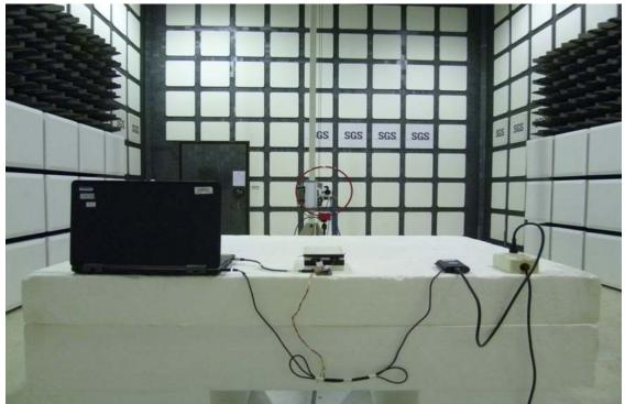
Radiated Emission Set up Photos (Below 1GHz)
