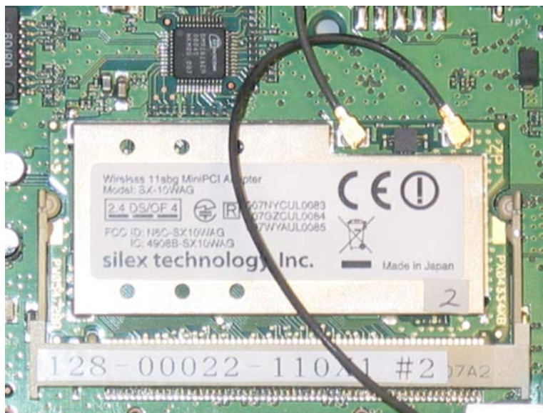
RF Module Installed
