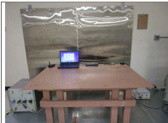
AC Line Conducted Emissions – Front View
