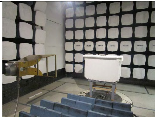
Radiated Emissions (>1GHz) – Rear View
