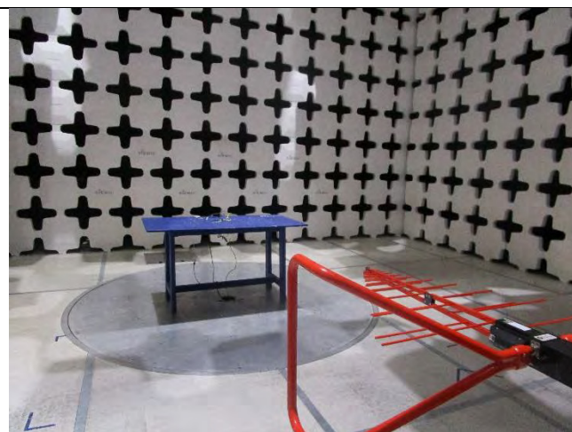
Radiated Emissions (<1GHz) – Rear View
