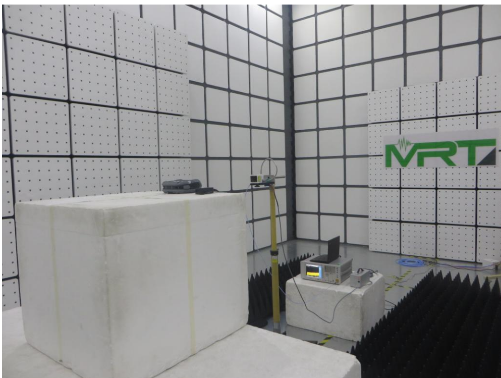
Description: Radiated Emission Test Setup for 18GHz ~ 40GHz (Host Model: RP4D)
