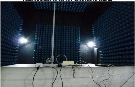
Radiated Emission Set up Photos (Below 1GHz)
