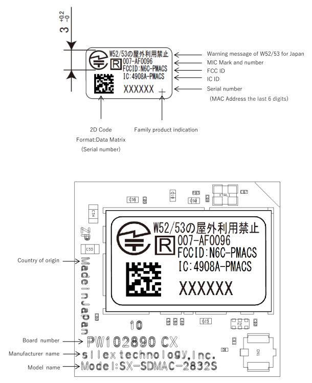
The Label is placed on the RF shielding case.
