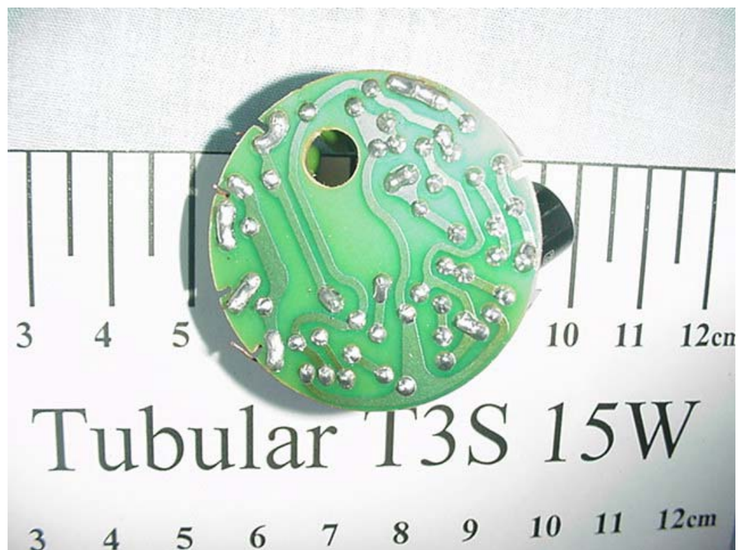
FIGURE 12 ENERGY SAVING LAMP (M/N: TUBULAR T3S 15W) MAIN BOARD (SOLDERED SIDE)
