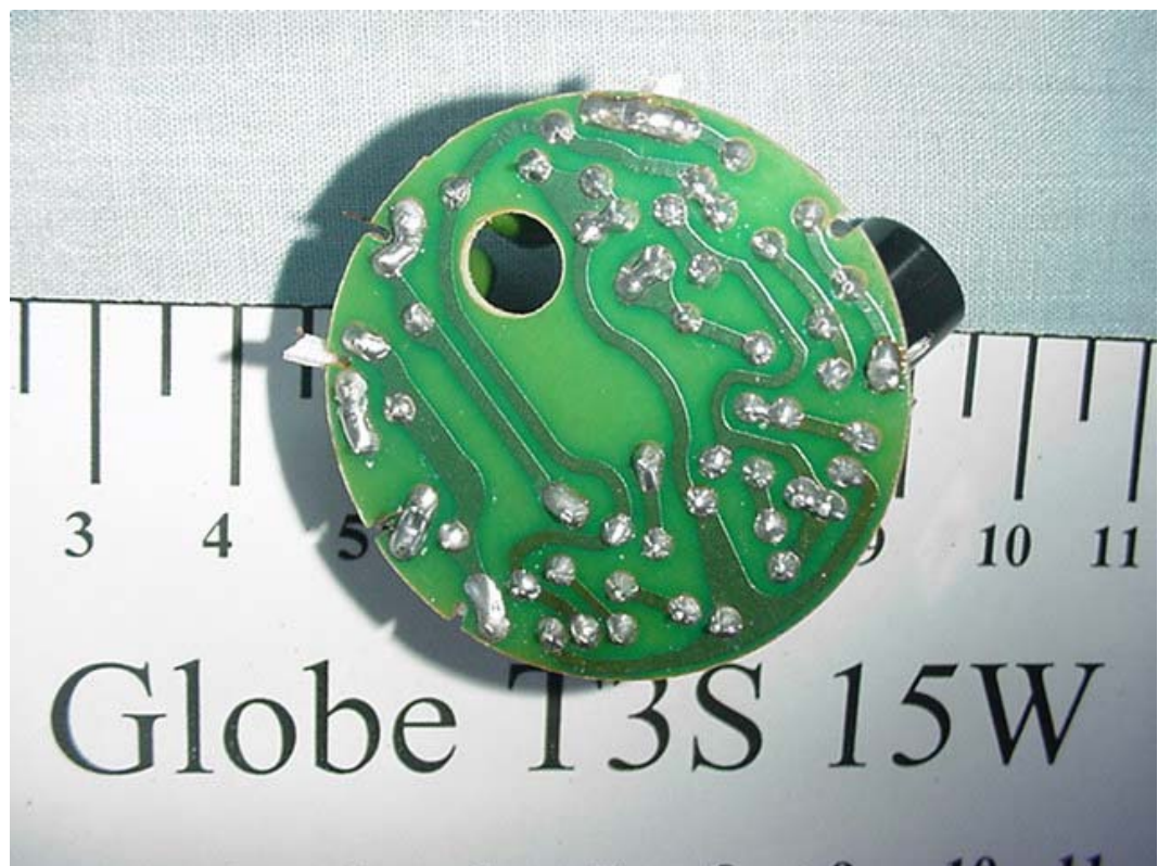
FIGURE 9 ENERGY SAVING LAMP (M/N: GLOBE T3S 15W) MAIN BOARD (SOLDERED SIDE)
