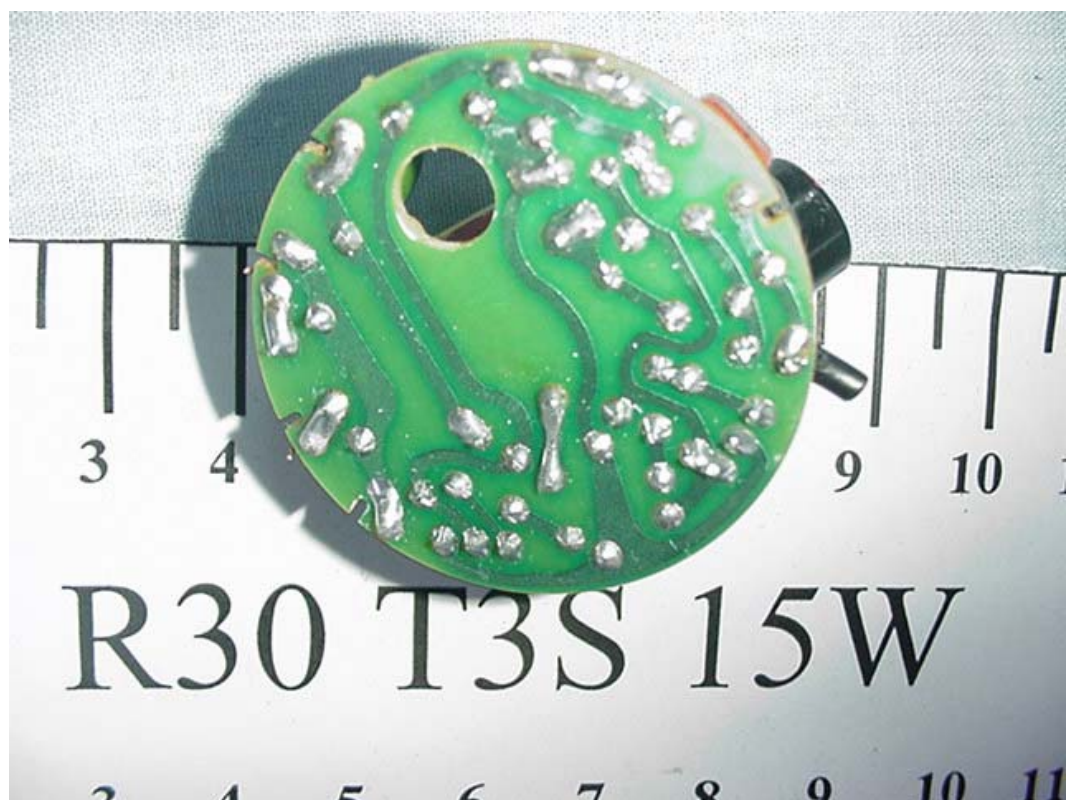
FIGURE 3 ENERGY SAVING LAMP (M/N: R30 T3S 15W) MAIN BOARD (SOLDERED SIDE)
