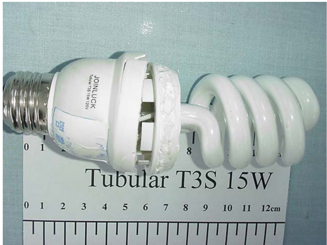
FIGURE 10 ENERGY SAVING LAMP (M/N: TUBULAR T3S 15W) COVER REMOVED
