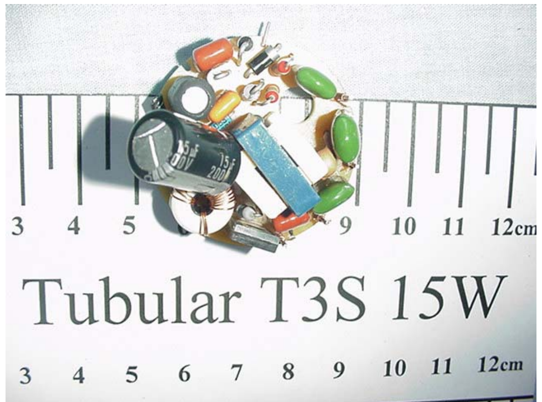
FIGURE 11 ENERGY SAVING LAMP (M/N: TUBULAR T3S 15W) MAIN BOARD (COMPONENT SIDE)
