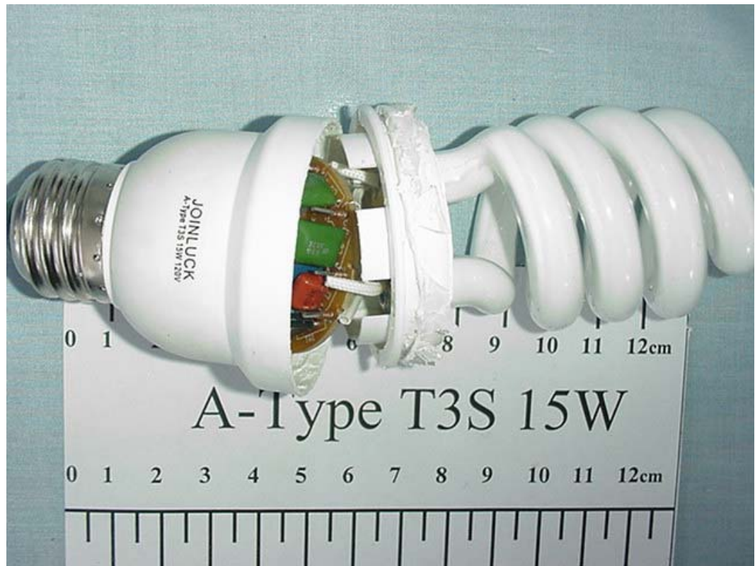
FIGURE 4 ENERGY SAVING LAMP (M/N: A-TYPE T3S 15W) COVER REMOVED
