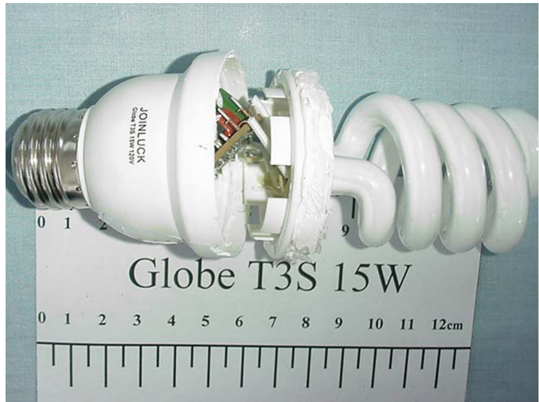
FIGURE 7 ENERGY SAVING LAMP (M/N: GLOBE T3S 15W) COVER REMOVED
