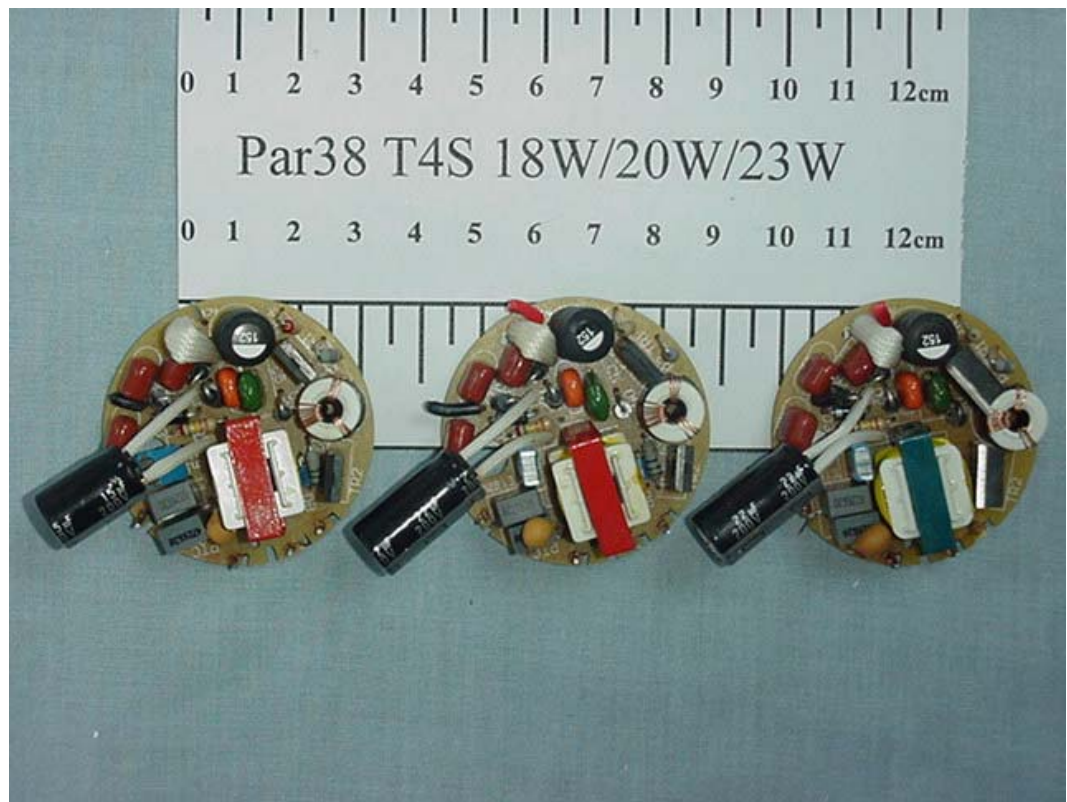
FIGURE 2 ENERGY SAVING LAMP (M/N: PAR38 T4S 18W/20W/23W) MAIN BOARD (COMPONENT SIDE)
