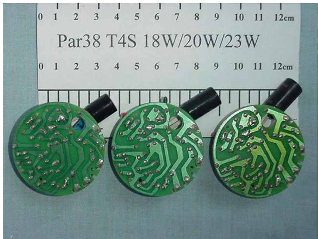
FIGURE 3 ENERGY SAVING LAMP (M/N: PAR38 T4S 18W/20W/23W) MAIN BOARD (SOLDERED SIDE)
