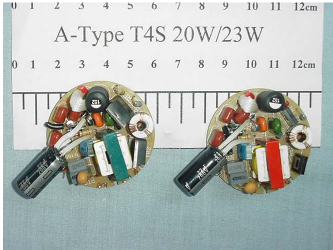
FIGURE 11 ENERGY SAVING LAMP (M/N: A-TYPE T4S 20W/23W) MAIN BOARD (COMPONENT SIDE)
