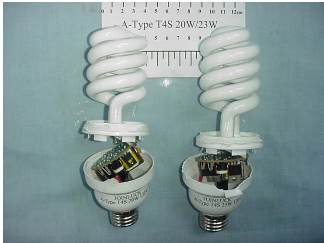
FIGURE 10 ENERGY SAVING LAMP (M/N: A-TYPE T4S 20W/23W) COVER REMOVED
