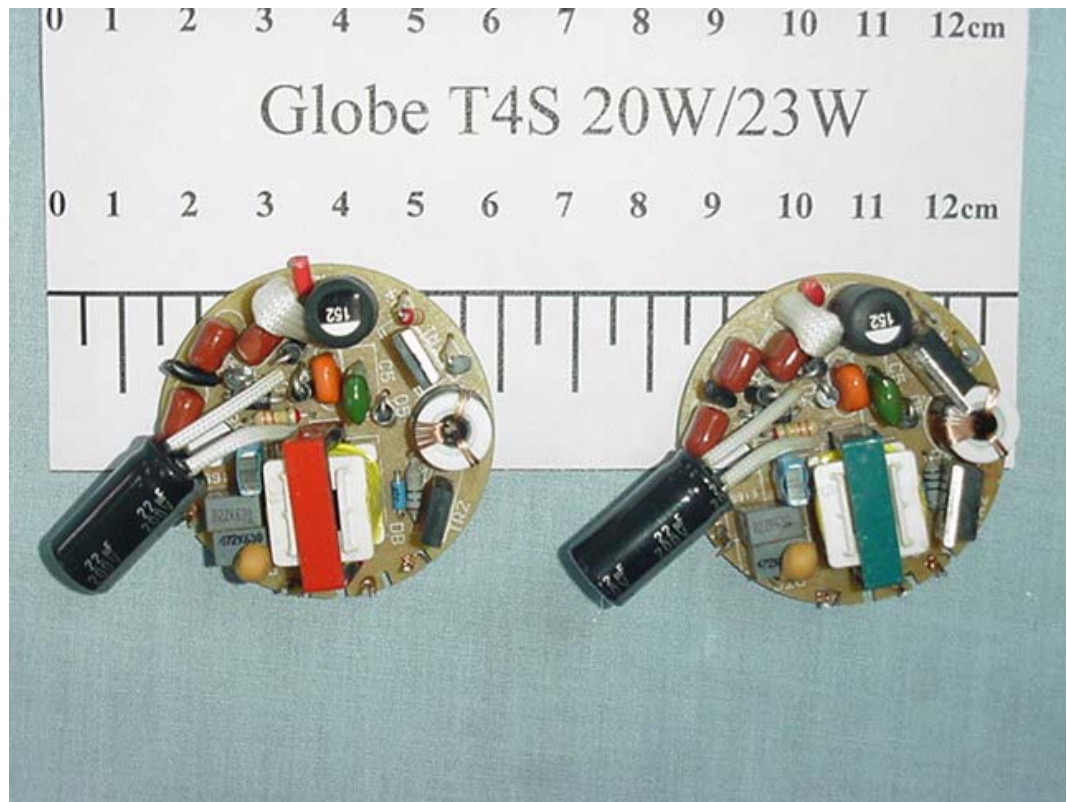
FIGURE 8 ENERGY SAVING LAMP (M/N: GLOBE T4S 20W/23W) MAIN BOARD (COMPONENT SIDE)
