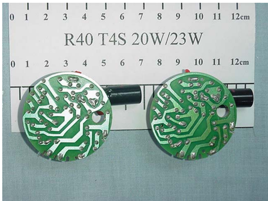
FIGURE 6 ENERGY SAVING LAMP (M/N: M/N: R40 T4S 20W/23W) MAIN BOARD (SOLDERED SIDE)
