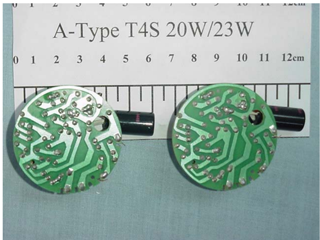
FIGURE 12 ENERGY SAVING LAMP (M/N: A-TYPE T4S 20W/23W) MAIN BOARD (SOLDERED SIDE)
