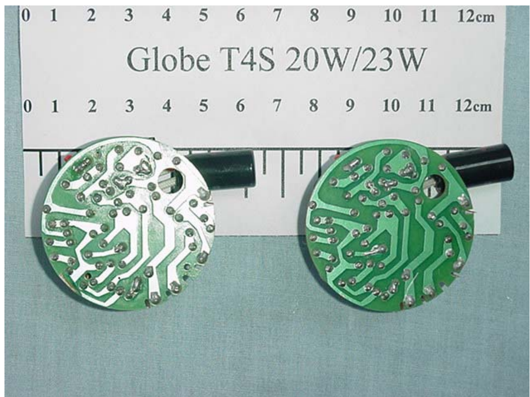
FIGURE 9 ENERGY SAVING LAMP (M/N: GLOBE T4S 20W/23W) MAIN BOARD (SOLDERED SIDE)
