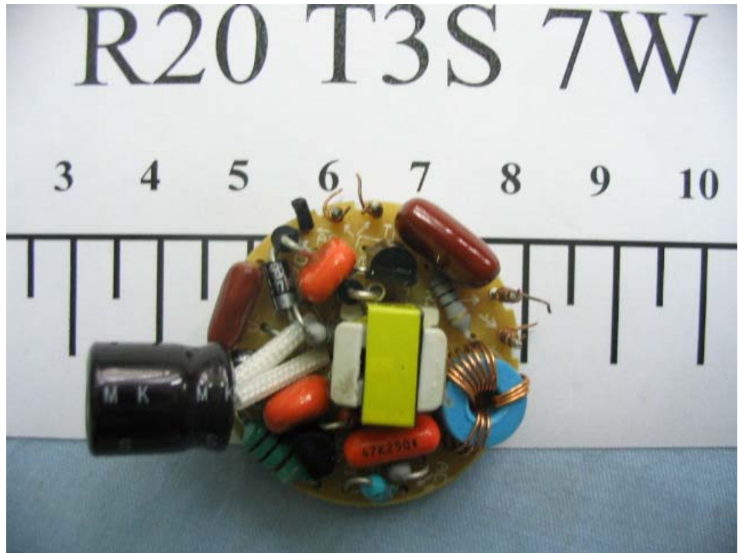
FIGURE 11 ENERGY SAVING LAMP (M/N: R20 T3S 7W) MAIN BOARD (COMPONENT SIDE)
