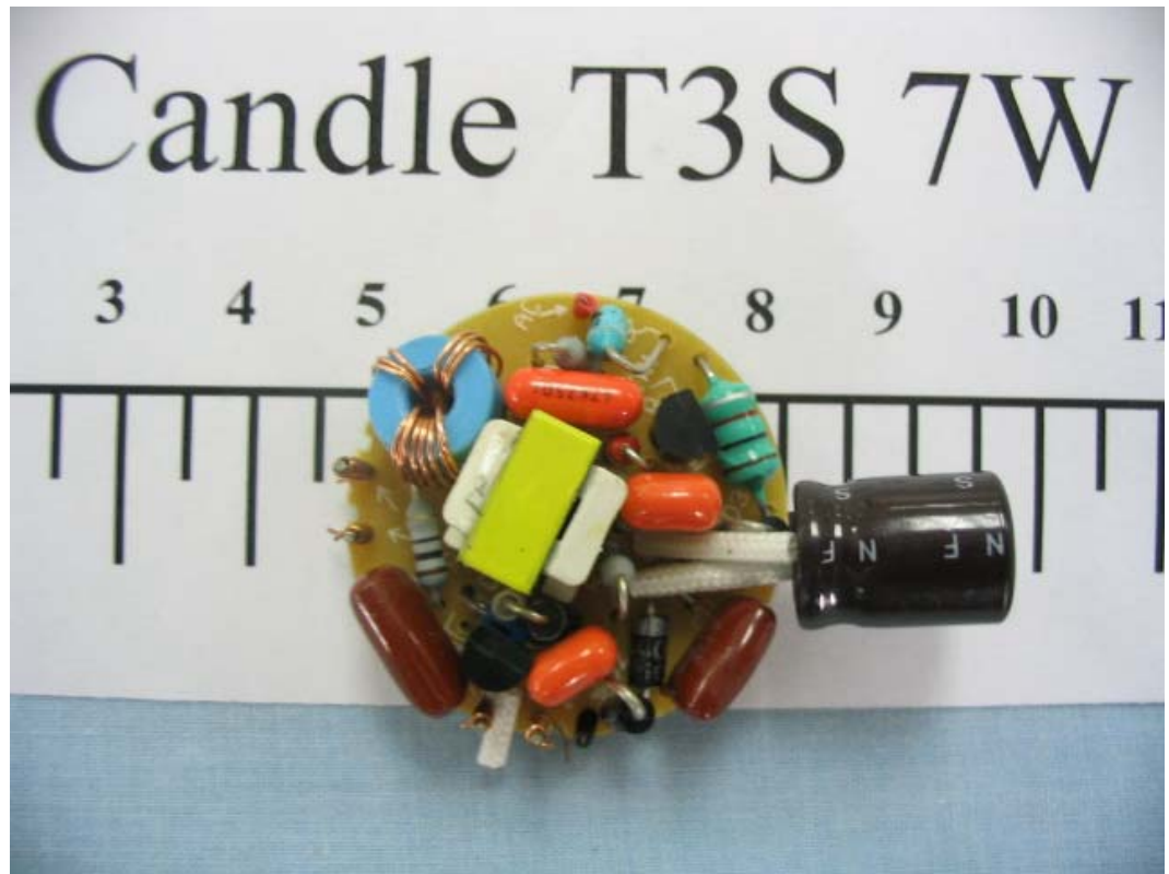
FIGURE 7 ENERGY SAVING LAMP (M/N: CANDLE T3S 7W) MAIN BOARD (COMPONENT SIDE)
