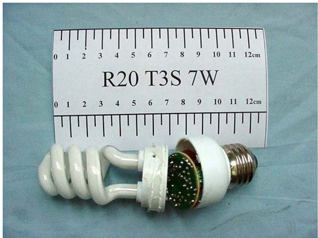
FIGURE 10 ENERGY SAVING LAMP (M/N: R20 T3S 7W) COVER REMOVED 2
