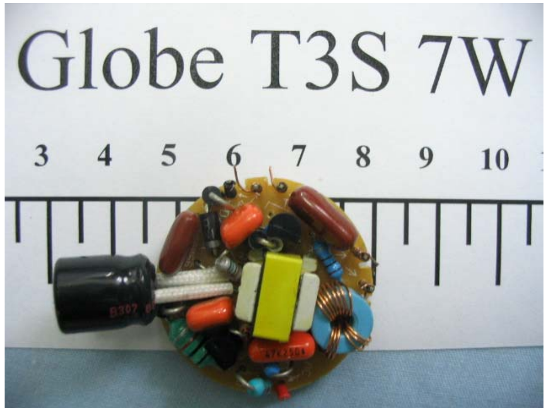
FIGURE 3 ENERGY SAVING LAMP (M/N: GLOBE T3S 7W) MAIN BOARD (COMPONENT SIDE)
