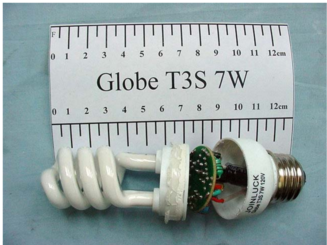
FIGURE 2 ENERGY SAVING LAMP (M/N: GLOBE T3S 7W) COVER REMOVED 2
