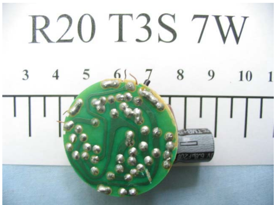
FIGURE 12 ENERGY SAVING LAMP (M/N: R20 T3S 7W) MAIN BOARD (SOLDERED SIDE)
