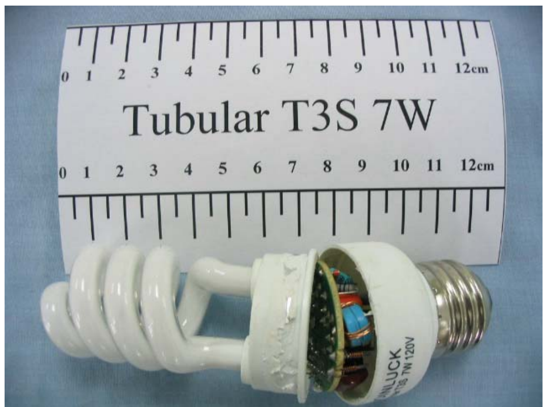
FIGURE 14 ENERGY SAVING LAMP (M/N: TUBULAR T3S 7W) COVER REMOVED 2
