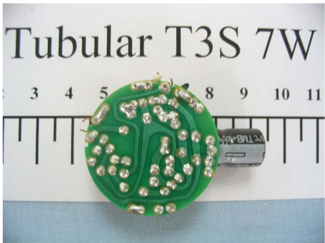
FIGURE 16 ENERGY SAVING LAMP (M/N: TUBULAR T3S 7W) MAIN BOARD (SOLDERED SIDE)
