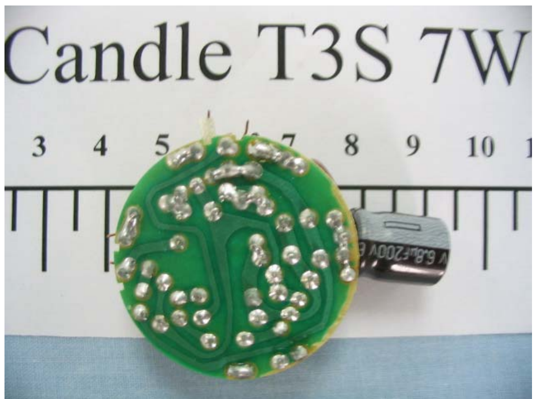
FIGURE 8 ENERGY SAVING LAMP (M/N: CANDLE T3S 7W) MAIN BOARD (SOLDERED SIDE)
