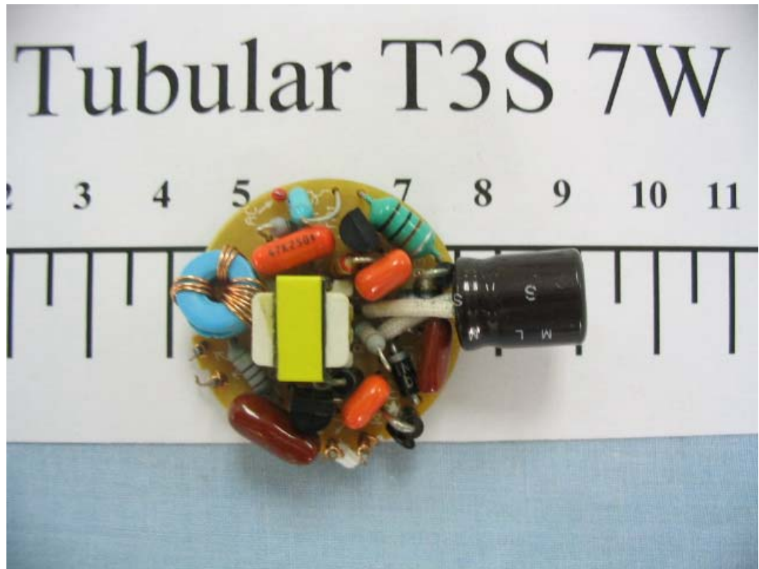
FIGURE 15 ENERGY SAVING LAMP (M/N: TUBULAR T3S 7W) MAIN BOARD (COMPONENT SIDE)
