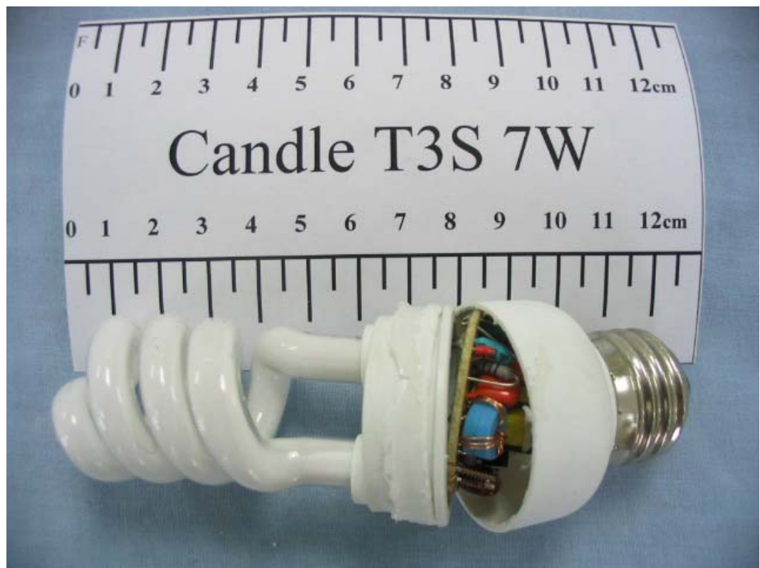
FIGURE 6 ENERGY SAVING LAMP (M/N: CANDLE T3S 7W) COVER REMOVED 2
