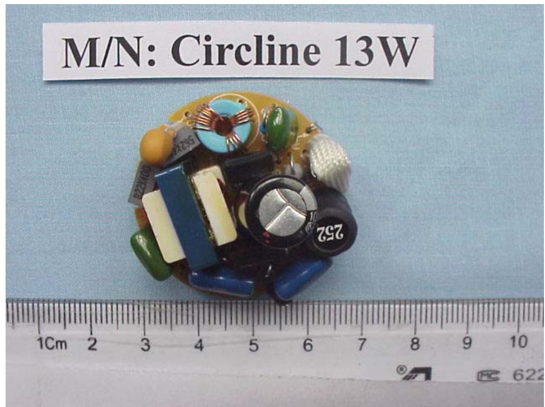
FIGURE 2 ENERGY SAVING LAMP (M/N: CIRCLINE 13W) MAIN BOARD (COMPONENT SIDE)
