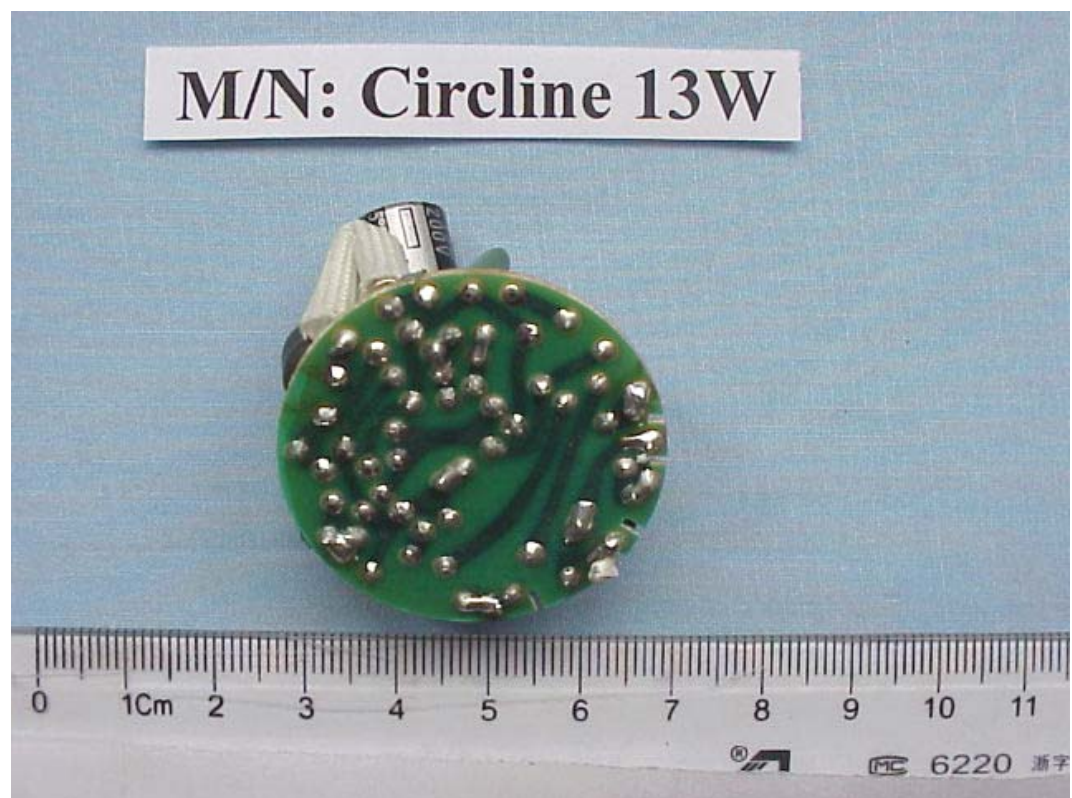
FIGURE 3 ENERGY SAVING LAMP (M/N: CIRCLINE 13W) MAIN BOARD (SOLDERED SIDE)
