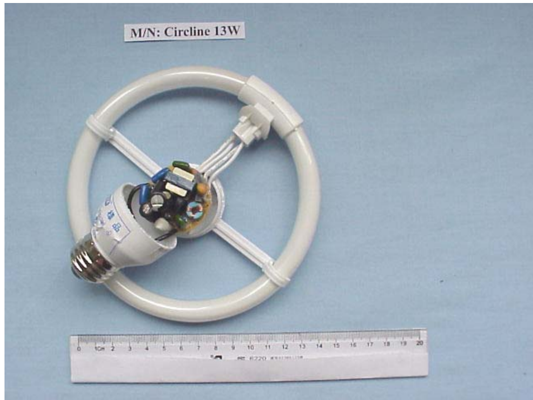
FIGURE 1 ENERGY SAVING LAMP (M/N: CIRCLINE 13W) COVER REMOVED
