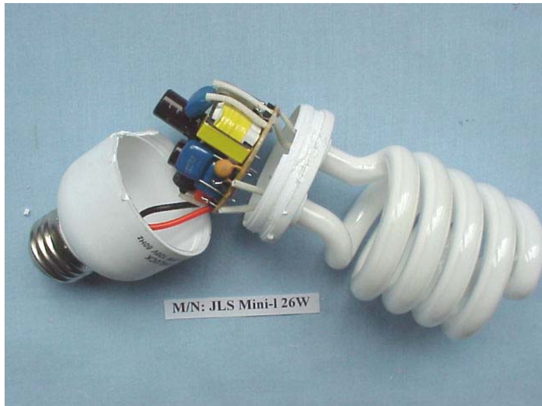
FIGURE 10 ENERGY SAVING LAMP (M/N: JLS MINI-I 26W) COVER REMOVED
