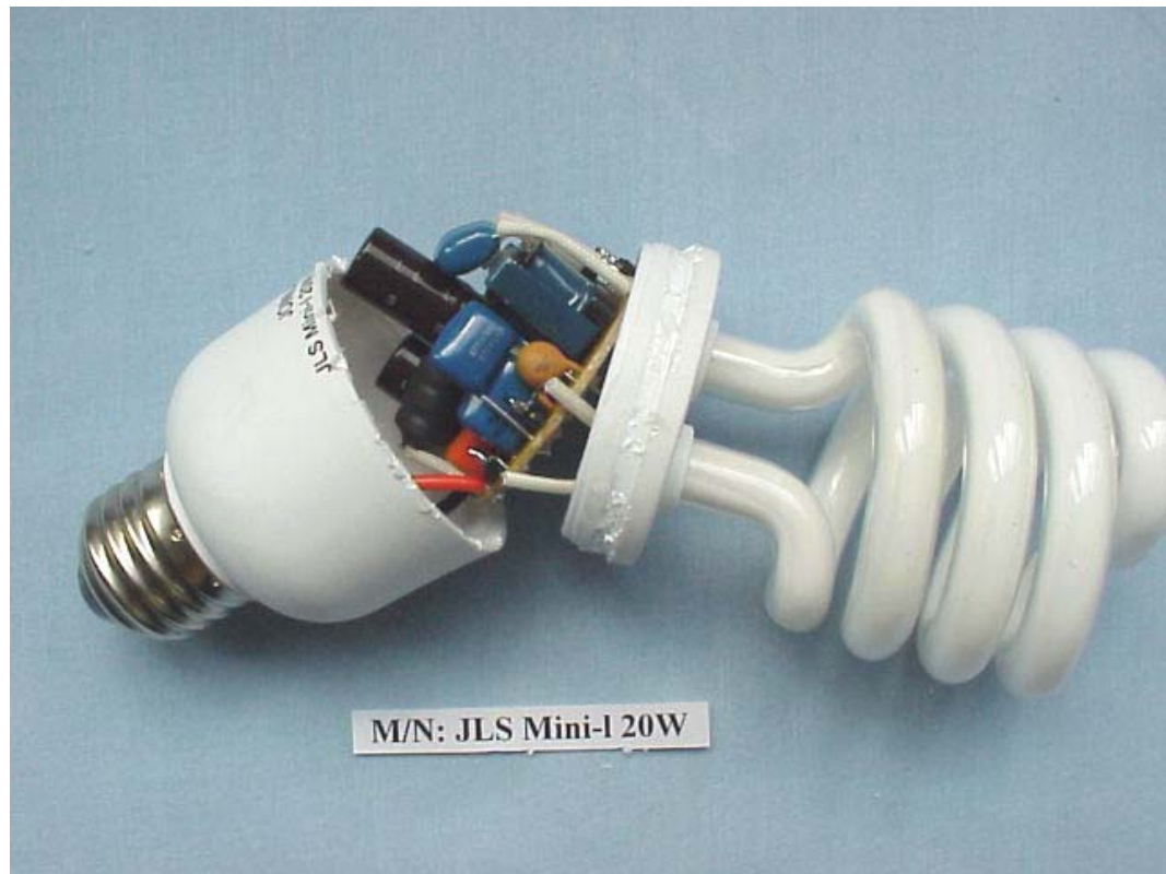
FIGURE 4 ENERGY SAVING LAMP (M/N: JLS MINI-I 20W) COVER REMOVED
