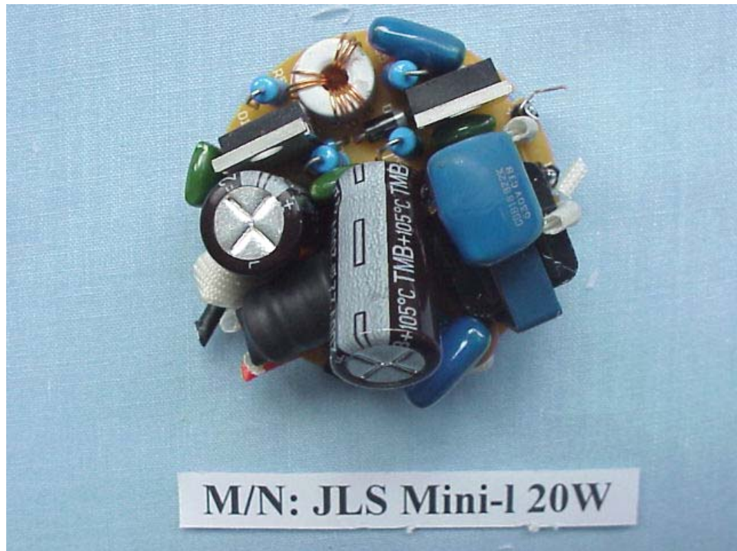
FIGURE 5 ENERGY SAVING LAMP (M/N: JLS MINI-I 20W) MAIN BOARD (COMPONENT SIDE)
