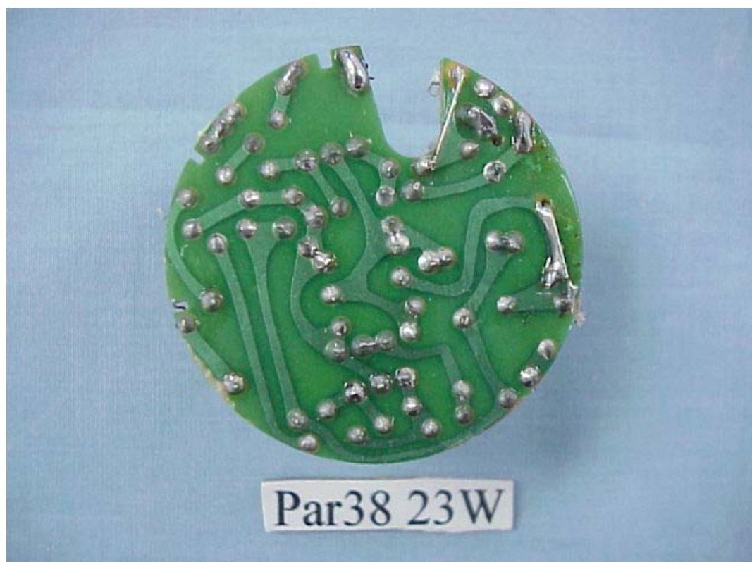
FIGURE 3 ENERGY SAVING LAMP (M/N: Par38 23W) MAIN BOARD (SOLDERED SIDE)
