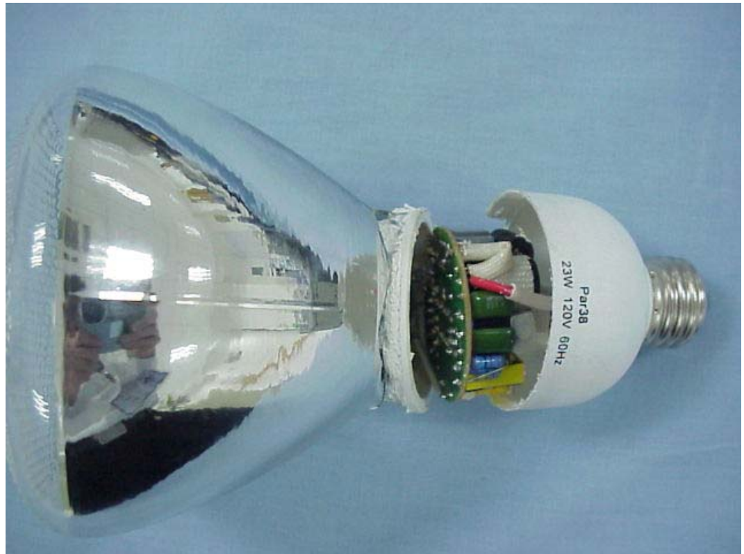
FIGURE 1 ENERGY SAVING LAMP (M/N: Par38 23W) COVER REMOVED
