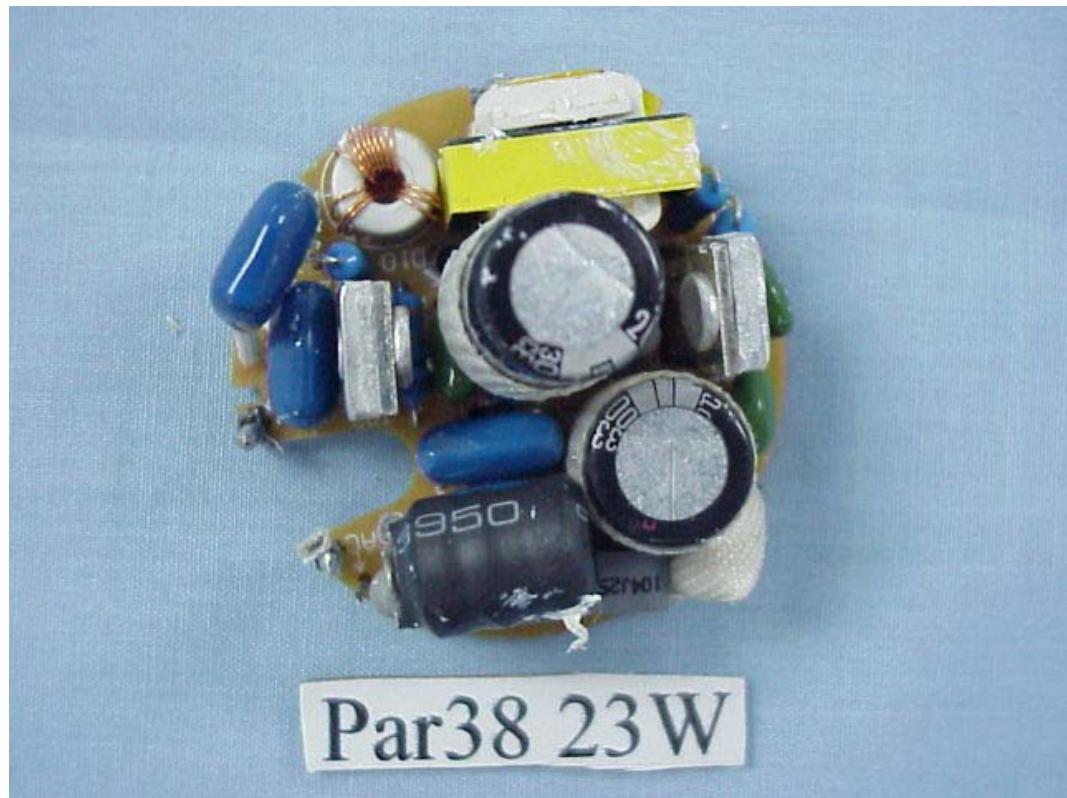
FIGURE 2 ENERGY SAVING LAMP (M/N: Par38 23W) MAIN BOARD (COMPONENT SIDE)
