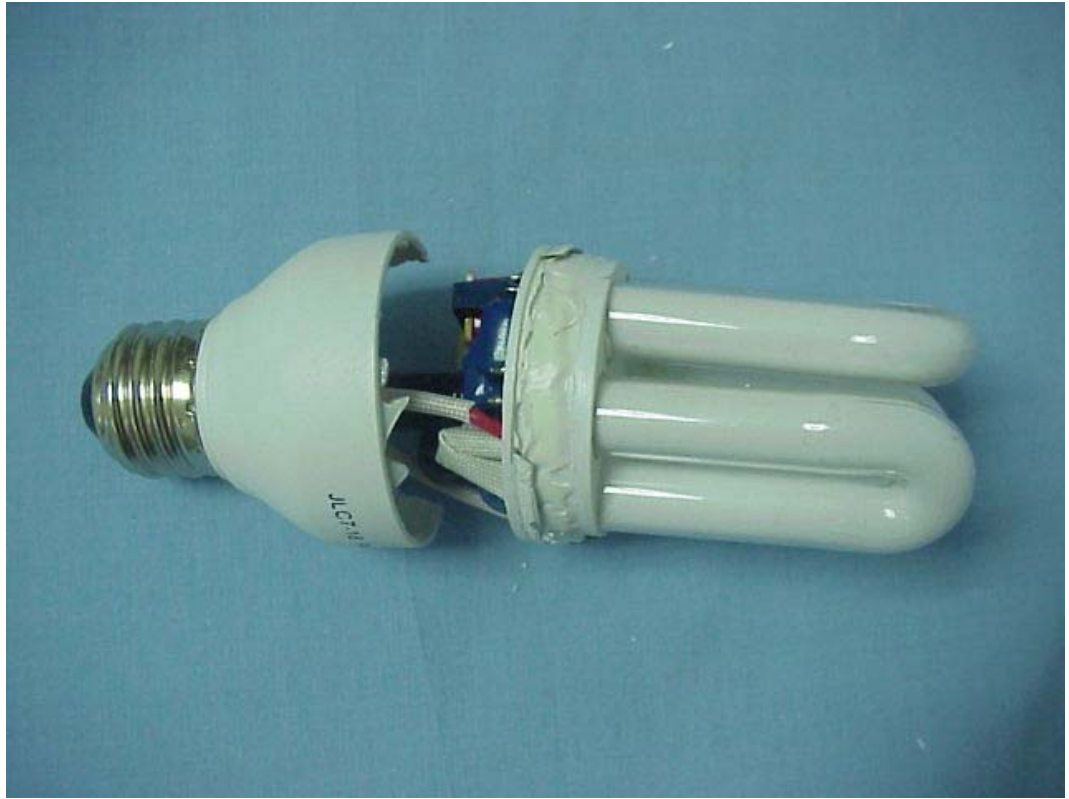
FIGURE 4 ELECTRONIC ENERGY SAVING LAMP (M/N: JLC7-18 REFLECTOR 11W) COVER REMOVED
