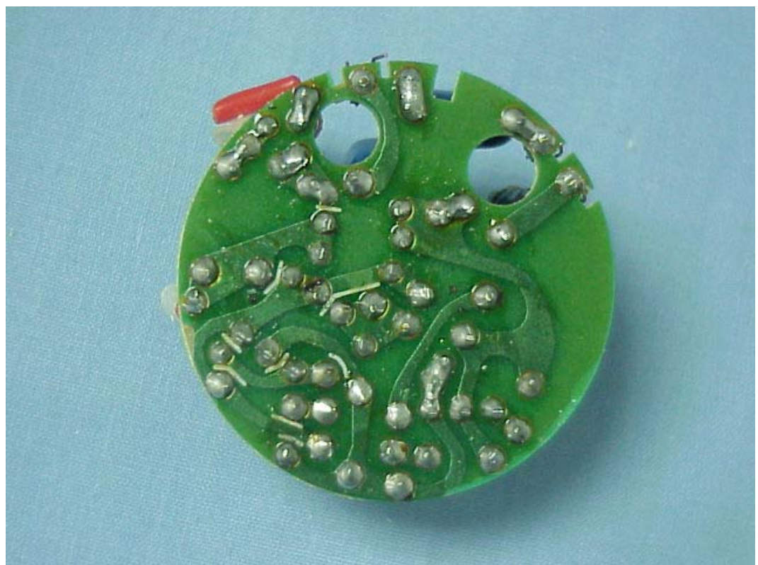
FIGURE 6 ELECTRONIC ENERGY SAVING LAMP (M/N: JLC7-18 REFLECTOR 11W) MAIN BOARD (SOLDERED SIDE)
