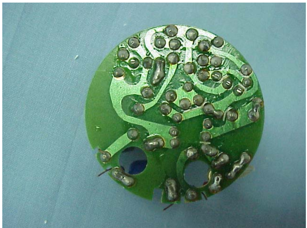
FIGURE 3 ELECTRONIC ENERGY SAVING LAMP (M/N: JLC7-18 A-TYPE 11W) MAIN BOARD (SOLDERED SIDE)
