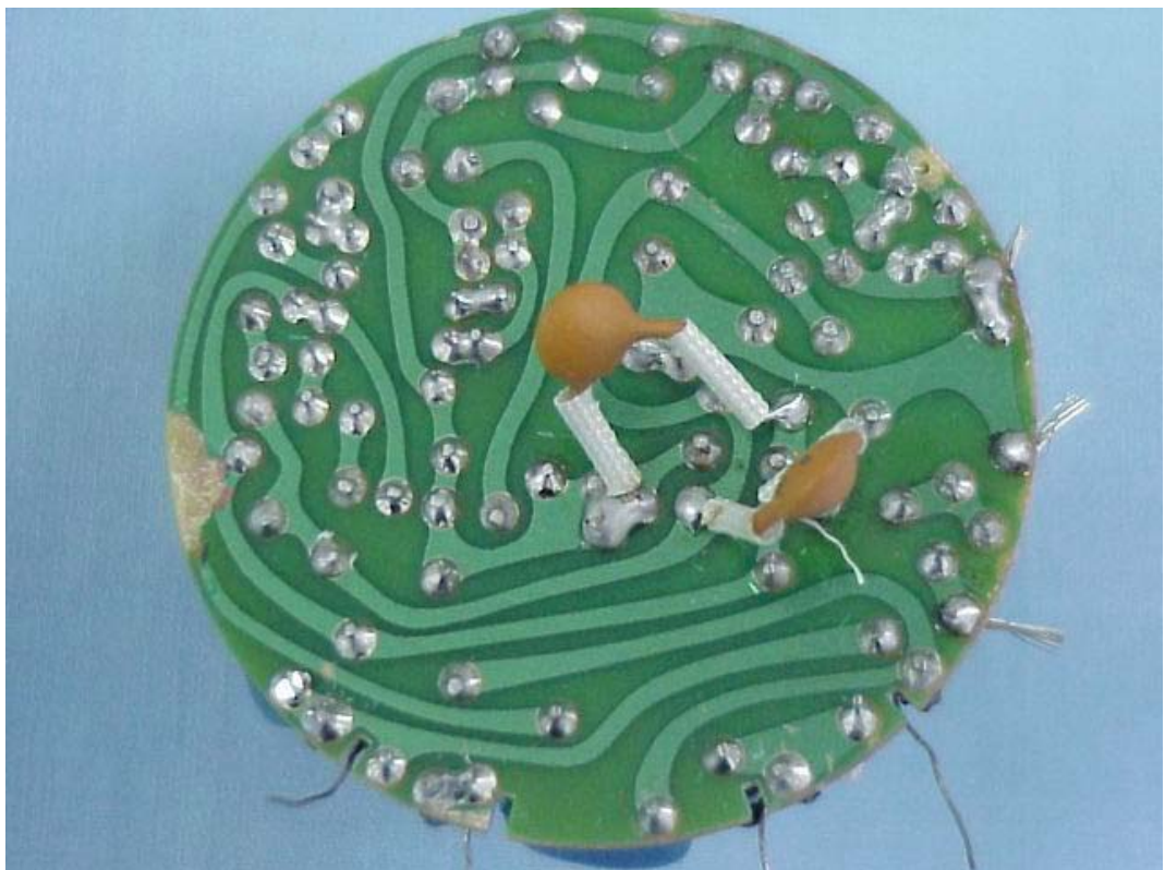
FIGURE 3 ELECTRONICS ENERGY SAVING LAMP (M/N: JLS 3-WAY 12W/20W/26W) MAIN BOARD (SOLDERED SIDE)
