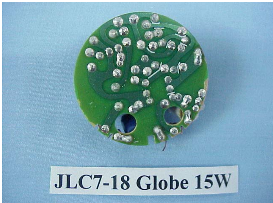
FIGURE 3 ELECTRONICS ENERGY SAVING LAMP (M/N: JLC7-18 GLOBE 15W) MAIN BOARD (SOLDERED SIDE)
