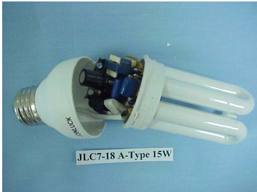
FIGURE 4 ELECTRONICS ENERGY SAVING LAMP (M/N: JLC7-18 A-TYPE 15W) COVER REMOVED
