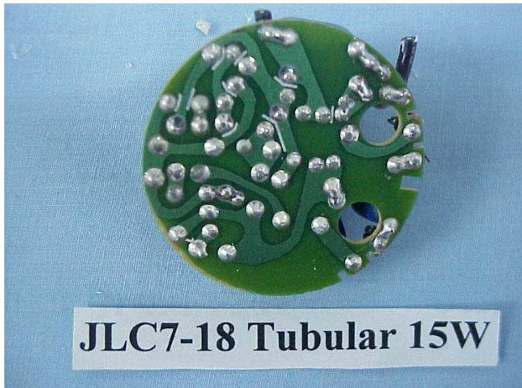
FIGURE 9 ELECTRONICS ENERGY SAVING LAMP (M/N: JLC7-18 TUBULAR 15W) MAIN BOARD (SOLDERED SIDE)
