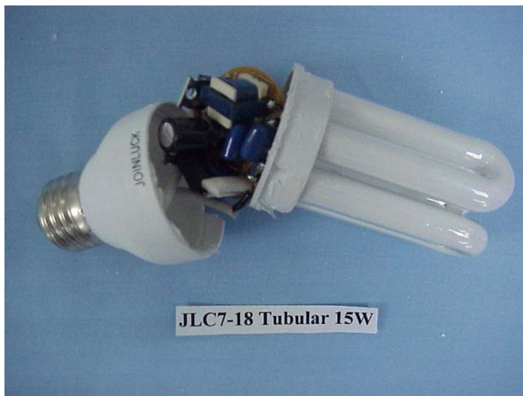
FIGURE 7 ELECTRONICS ENERGY SAVING LAMP (M/N: JLC7-18 TUBULAR 15W) COVER REMOVED
