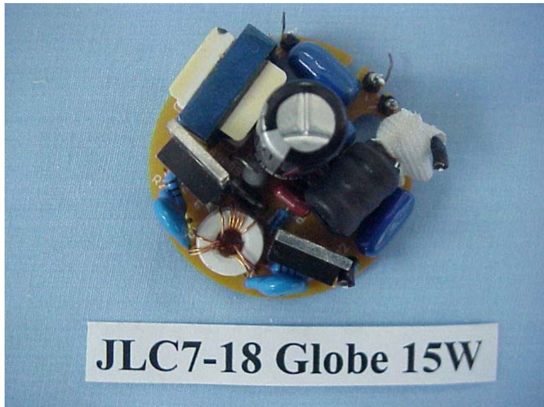
FIGURE 3 ELECTRONICS ENERGY SAVING LAMP (M/N: JLC7-18 GLOBE 15W) MAIN BOARD (SOLDERED SIDE)
