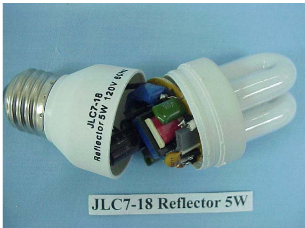
FIGURE 2 ELECTRONICS ENERGY SAVING LAMP (M/N: JLC7-18 REFLECTOR 5W) COVER REMOVED
