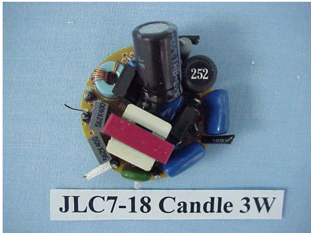
FIGURE 7 ELECTRONICS ENERGY SAVING LAMP (M/N: JLC7-18 CANDLE 3W) MAIN BOARD (COMPONENT SIDE)
