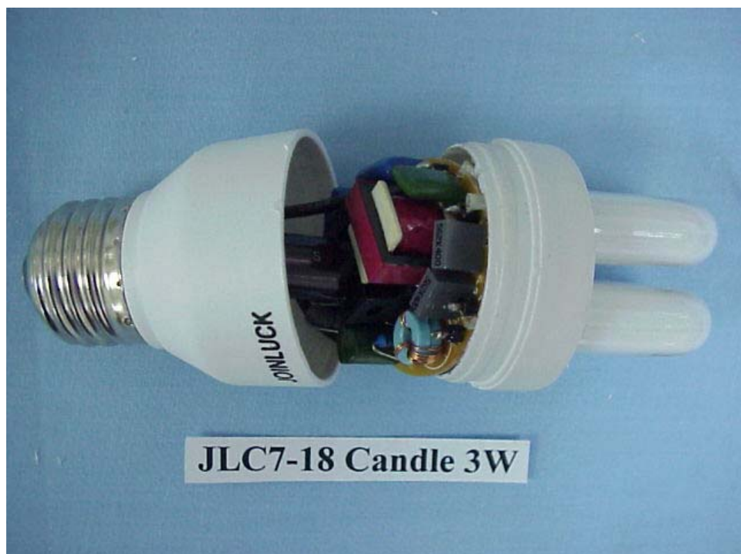
FIGURE 6 ELECTRONICS ENERGY SAVING LAMP (M/N: JLC7-18 CANDLE 3W) COVER REMOVED
