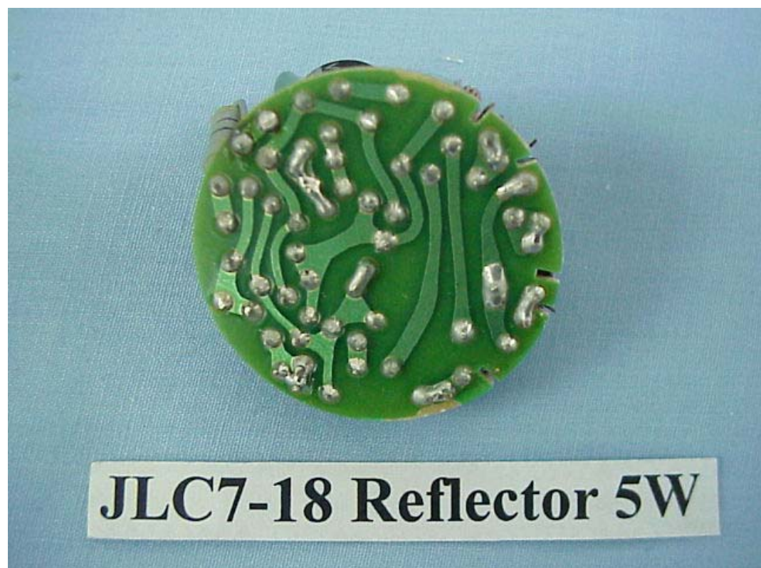
FIGURE 4 ELECTRONICS ENERGY SAVING LAMP (M/N: JLC7-18 REFLECTOR 5W) MAIN BOARD (SOLDERED SIDE)
