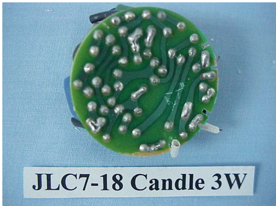
FIGURE 8 ELECTRONICS ENERGY SAVING LAMP (M/N: JLC7-18 CANDLE 3W) MAIN BOARD (SOLDERED SIDE)
