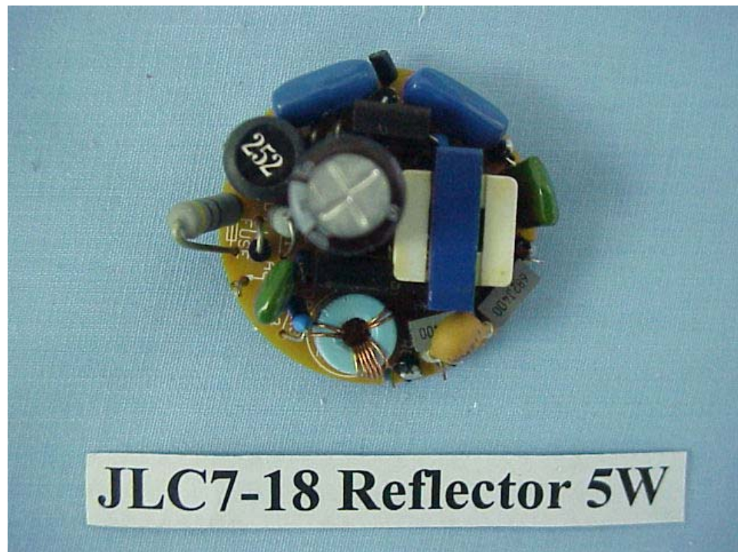
FIGURE 3 ELECTRONICS ENERGY SAVING LAMP (M/N: JLC7-18 REFLECTOR 5W) MAIN BOARD (COMPONENT SIDE)
