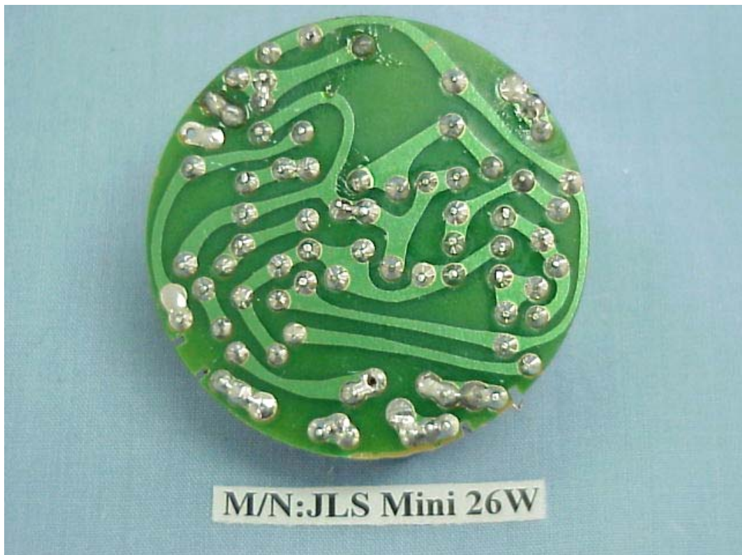
FIGURE 3 E.S.L (M/N: JLS Mini 26W) MAIN BOARD (SOLDERED SIDE)
