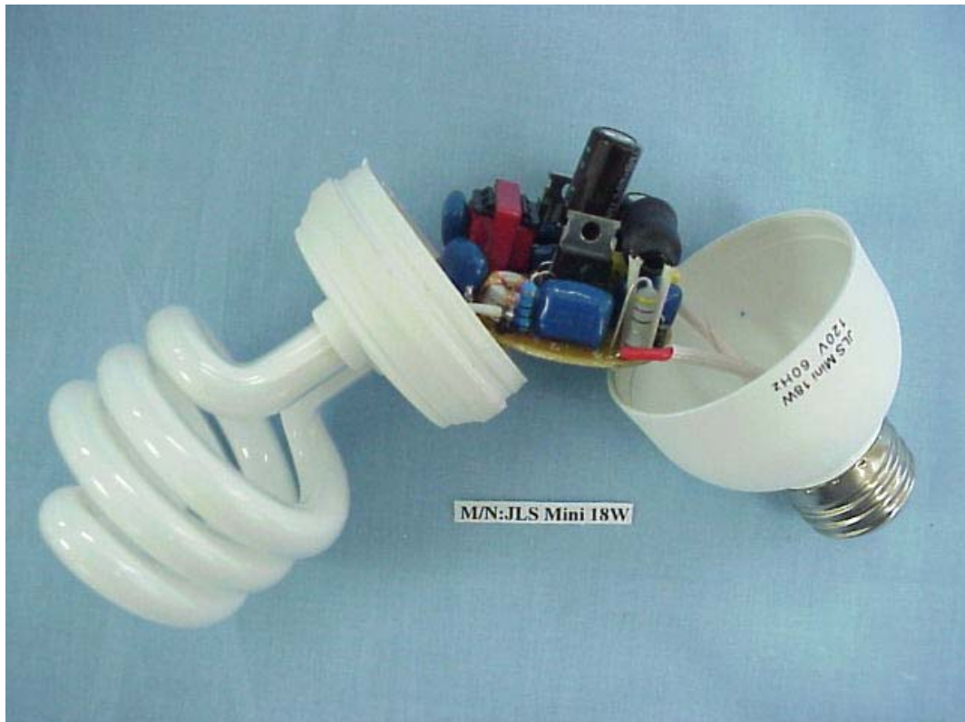
FIGURE 7 E.S.L (M/N: JLS Mini 18W) COVER REMOVED
