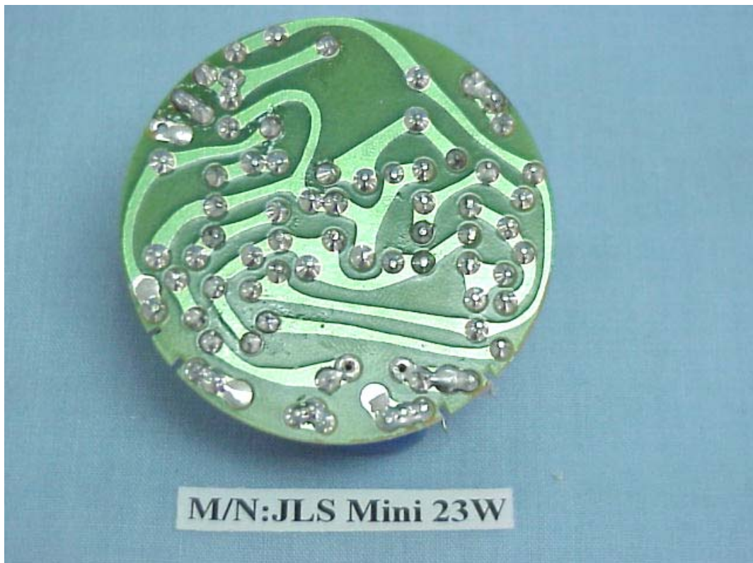
FIGURE 6 E.S.L (M/N: JLS Mini 23W) MAIN BOARD (SOLDERED SIDE)
