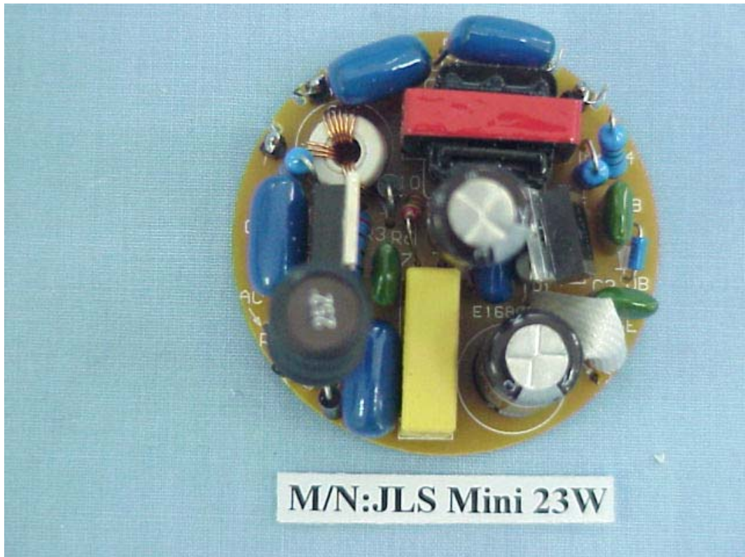
FIGURE 6 E.S.L (M/N: JLS Mini 23W) MAIN BOARD (SOLDERED SIDE)
