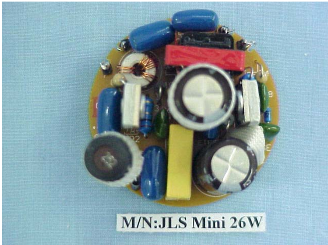
FIGURE 3 E.S.L (M/N: JLS Mini 26W) MAIN BOARD (SOLDERED SIDE)
