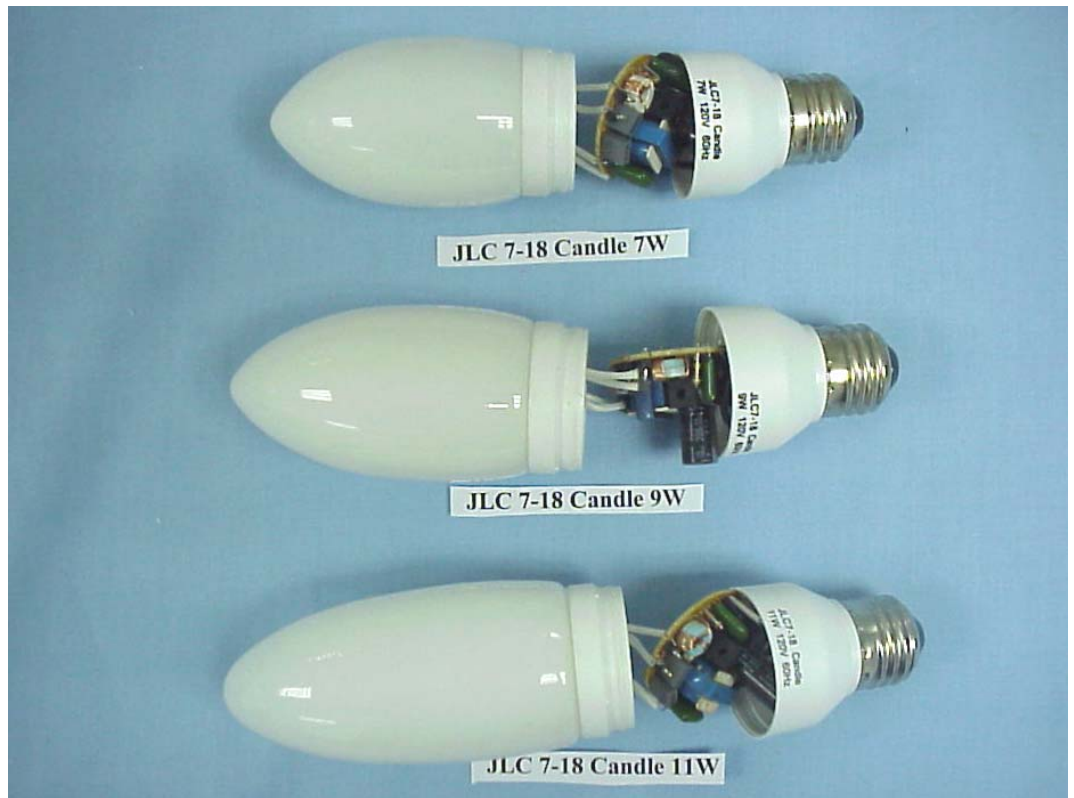
FIGURE 1 ELECTRONIC ENERGY SAVING LAMP (M/N: JLC 7-18 CANDLE 7W/9W/11W) COVER REMOVED
