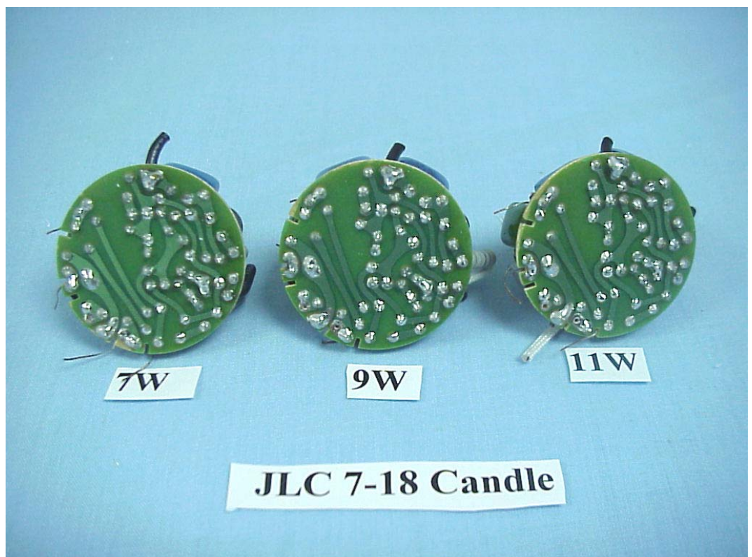
FIGURE 3 ELECTRONIC ENERGY SAVING LAMP (M/N: JLC 7-18 CANDLE 7W/9W/11W) MAIN BOARD (SOLDERED SIDE)
