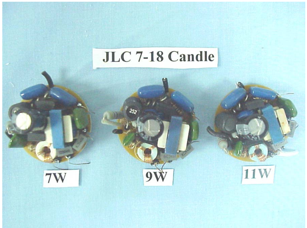
FIGURE 2 ELECTRONIC ENERGY SAVING LAMP (M/N: JLC 7-18 CANDLE 7W/9W/11W) MAIN BOARD (COMPONENT SIDE)
