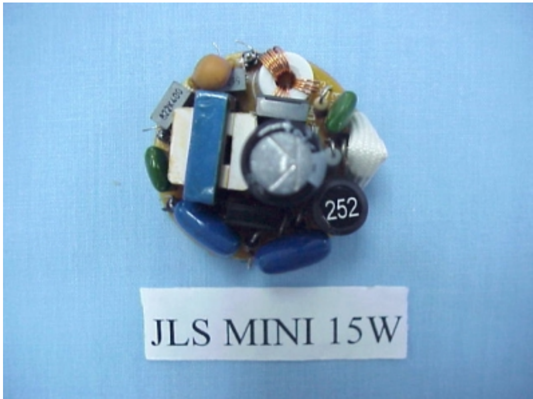
FIGURE 10 ENERGY SAVING LAMP (M/N: JLS MINI 15W) Main Board (Component Side)
