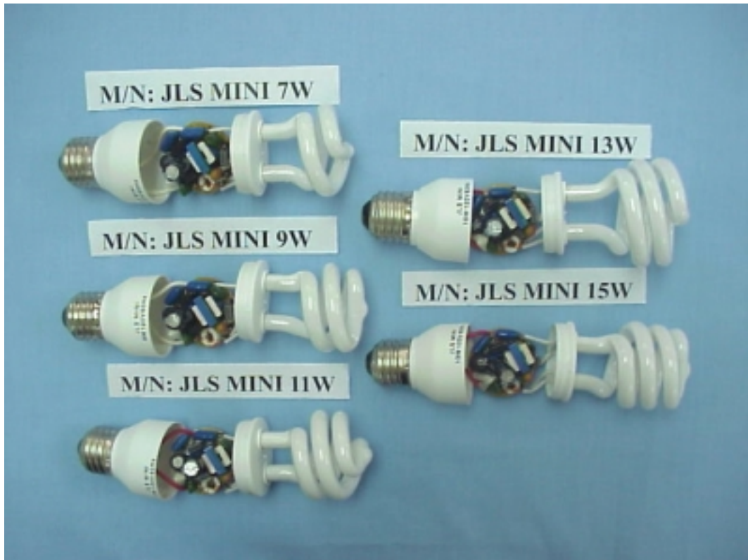
FIGURE 1 ENERGY SAVING LAMP (M/N: JLS MINI SERIALS) COVER REMOVED
