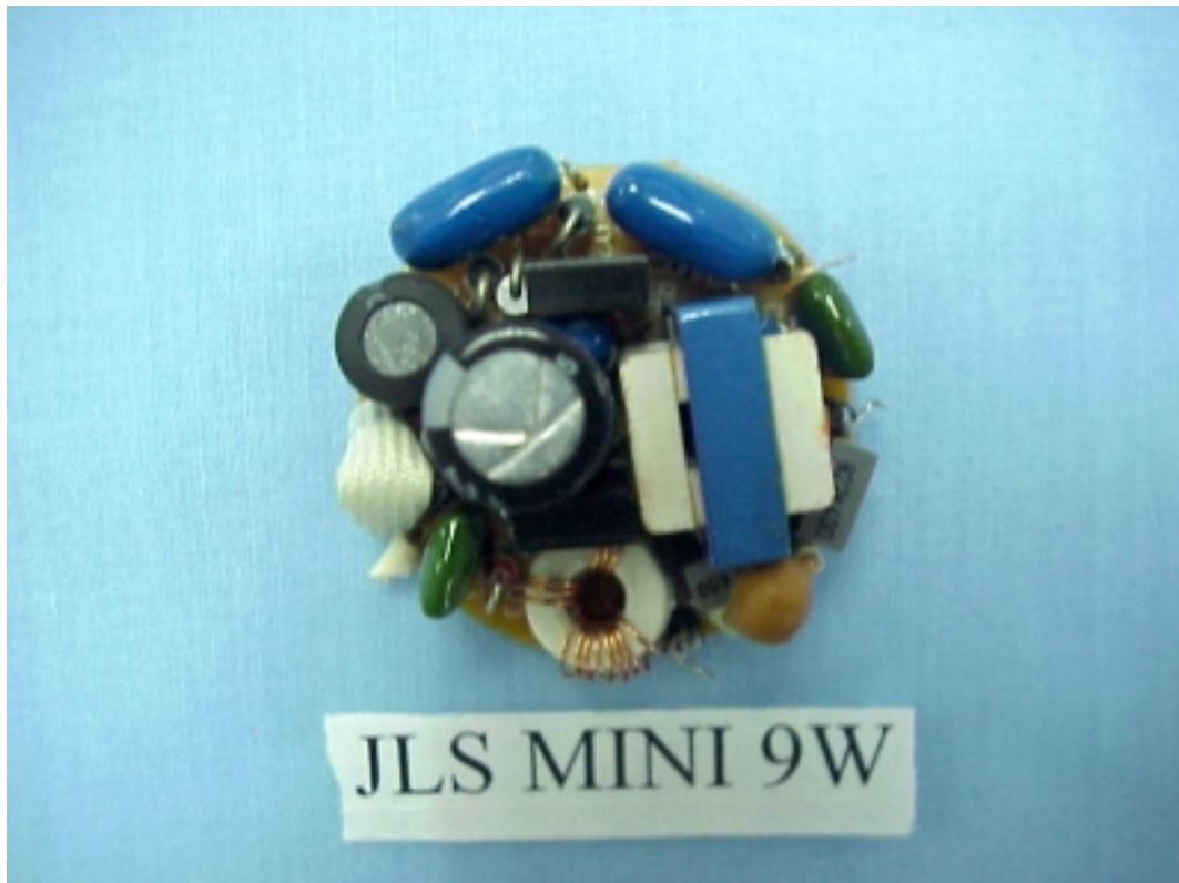
FIGURE 4 ENERGY SAVING LAMP (M/N: JLS MINI 9W) MAIN BOARD (COMPONENT SIDE)
