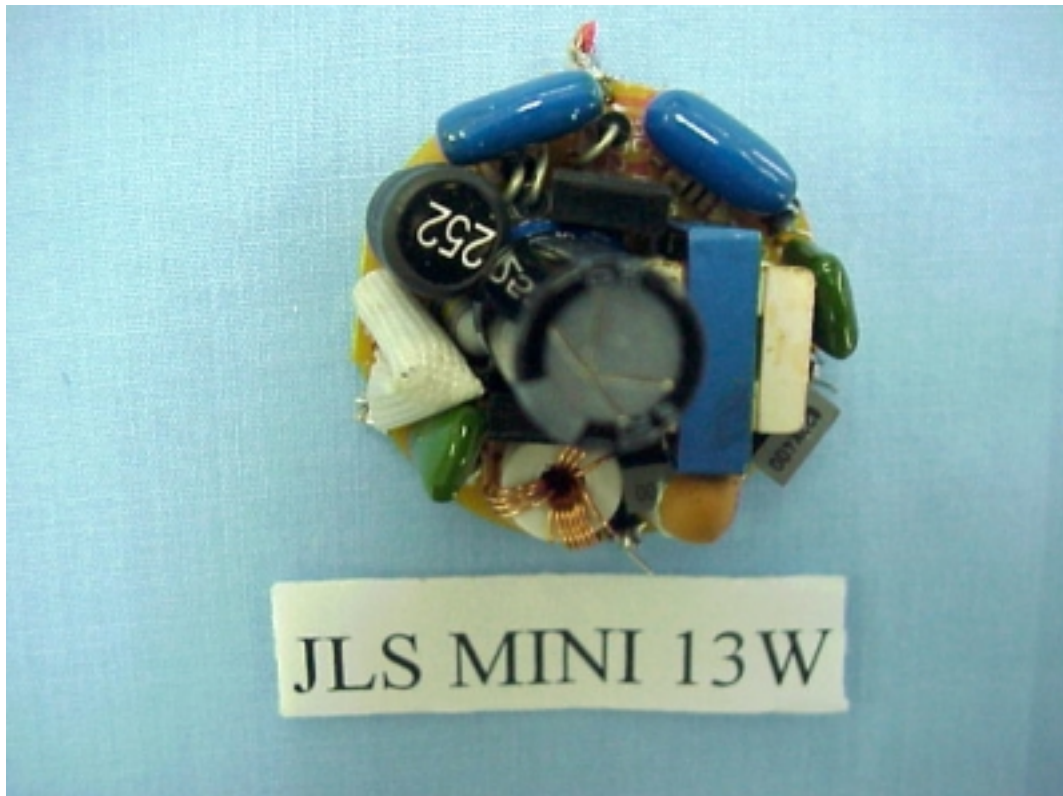
FIGURE 8 ENERGY SAVING LAMP (M/N: JLS MINI 13W) MAIN BOARD (COMPONENT SIDE)
