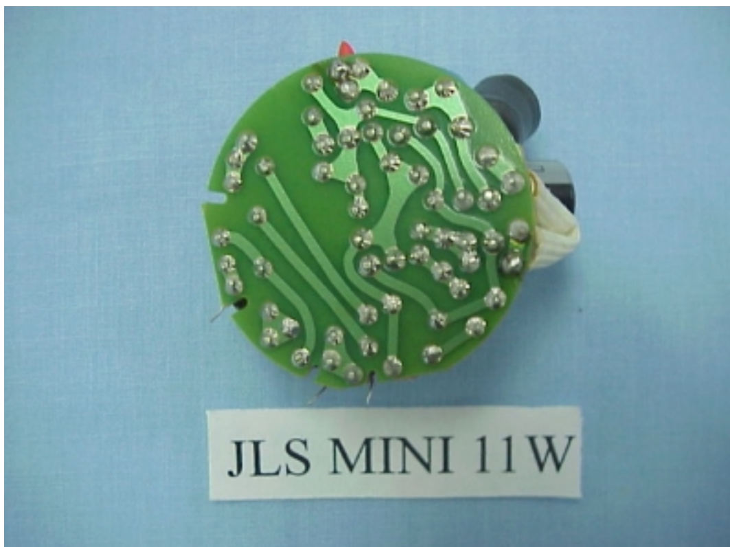
FIGURE 7 ENERGY SAVING LAMP (M/N: JLS MINI 11W) MAIN BOARD (SOLDERED SIDE)
