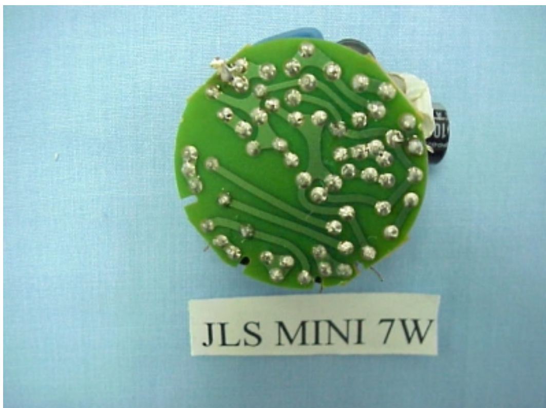
FIGURE 3 ENERGY SAVING LAMP (M/N: JLS MINI 7W) MAIN BOARD (SOLDERED SIDE)
