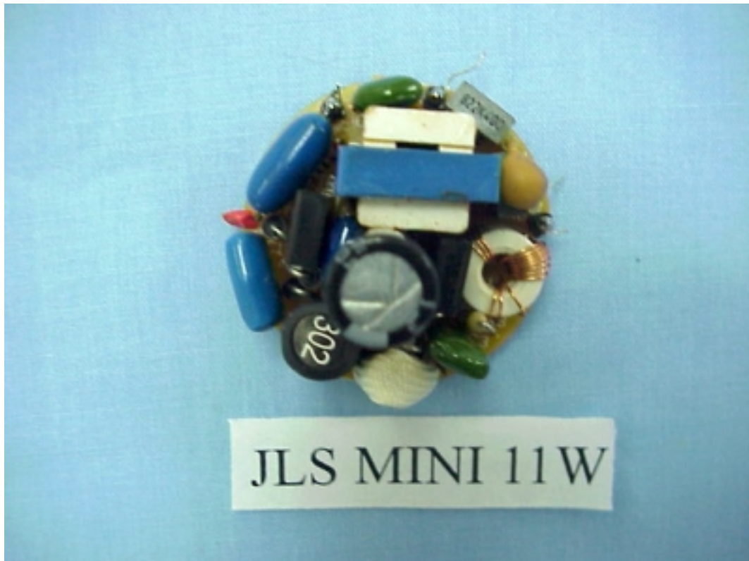
FIGURE 6 ENERGY SAVING LAMP (M/N: JLS MINI 11W) MAIN BOARD (COMPONENT SIDE)
