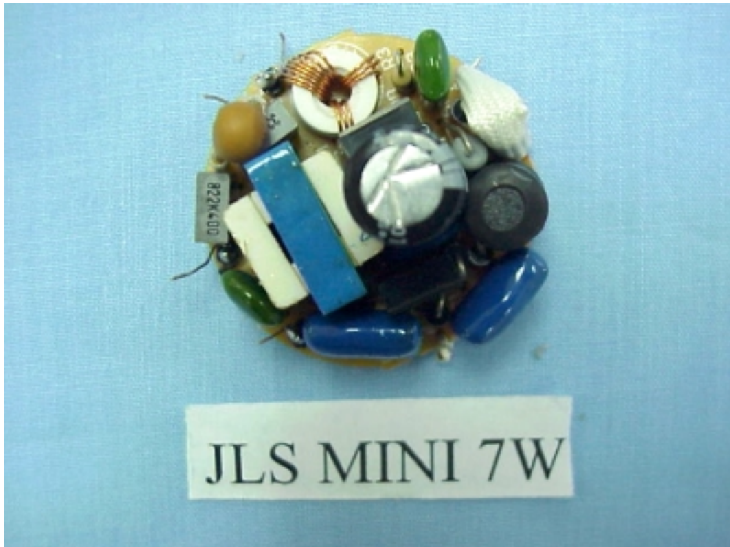
FIGURE 2 ENERGY SAVING LAMP (M/N: JLS MINI 7W) MAIN BOARD (COMPONENT SIDE)
