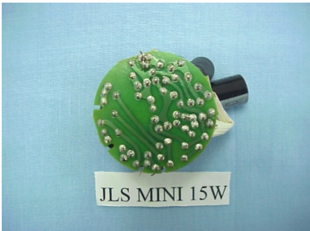
FIGURE 11 ENERGY SAVING LAMP (M/N: JLS MINI 15W) MAIN BOARD (SOLDERED SIDE)
