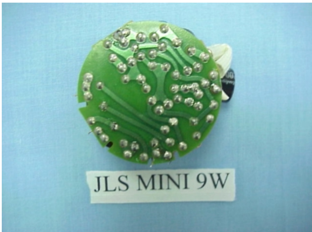
FIGURE 5 ENERGY SAVING LAMP (M/N: JLS MINI 9W) MAIN BOARD (SOLDERED SIDE)
