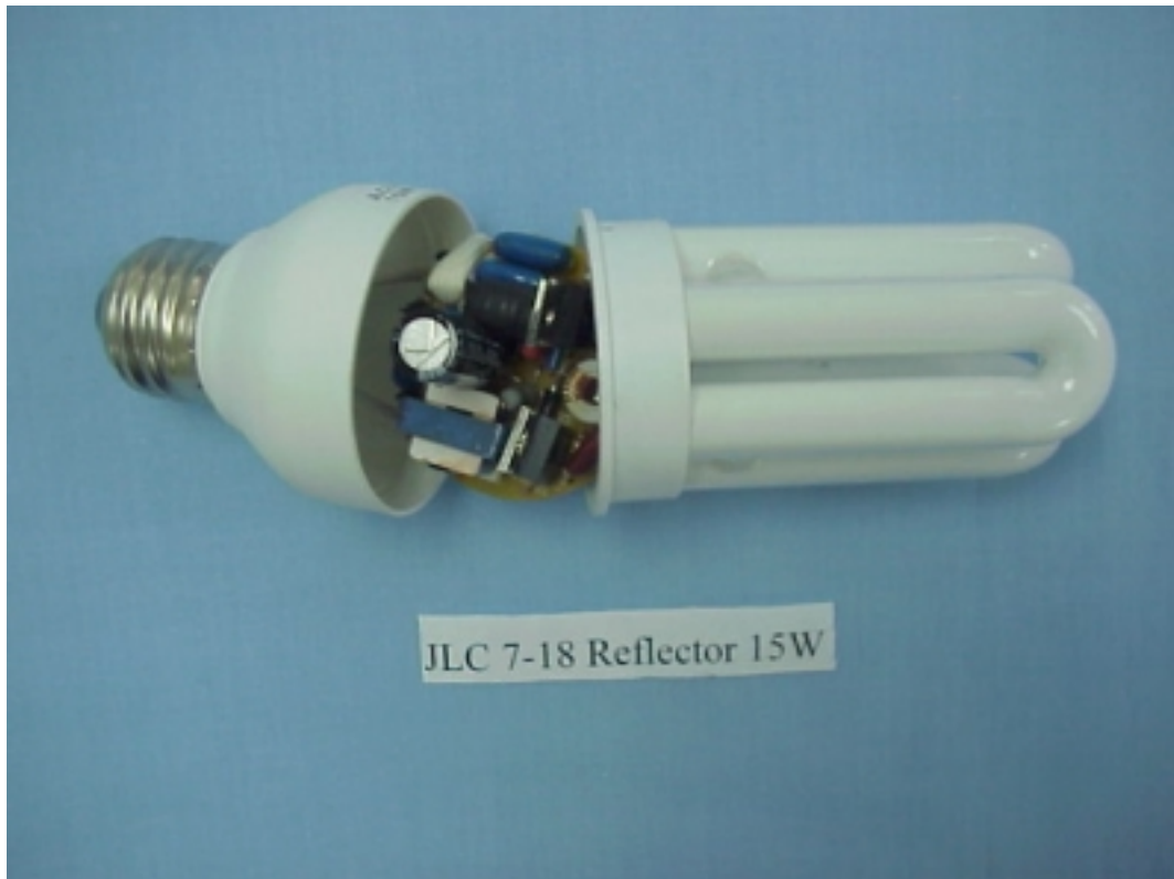
Figure 4 ENERGY SAVING LAMP (M/N: JLC 7-18 REFLECTOR 15W) COVER REMOVED
