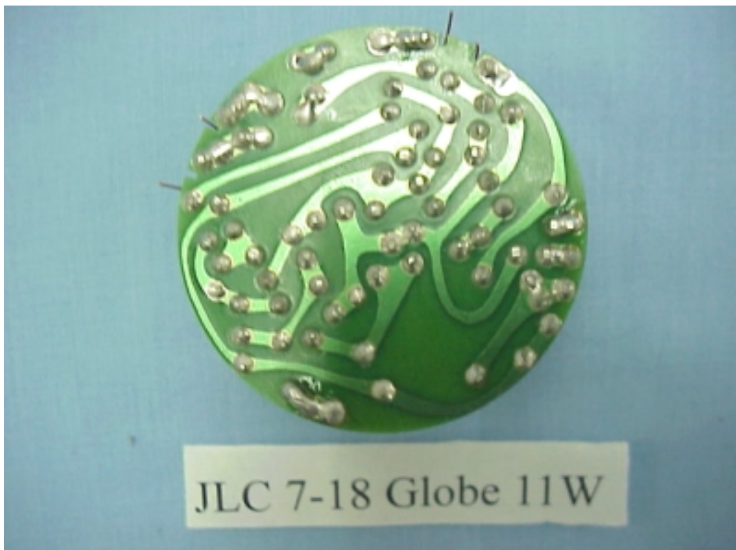
Figure 3 ENERGY SAVING LAMP (M/N: JLC 7-18 GLOBE 11W) MAIN BOARD (SOLDERED SIDE)
