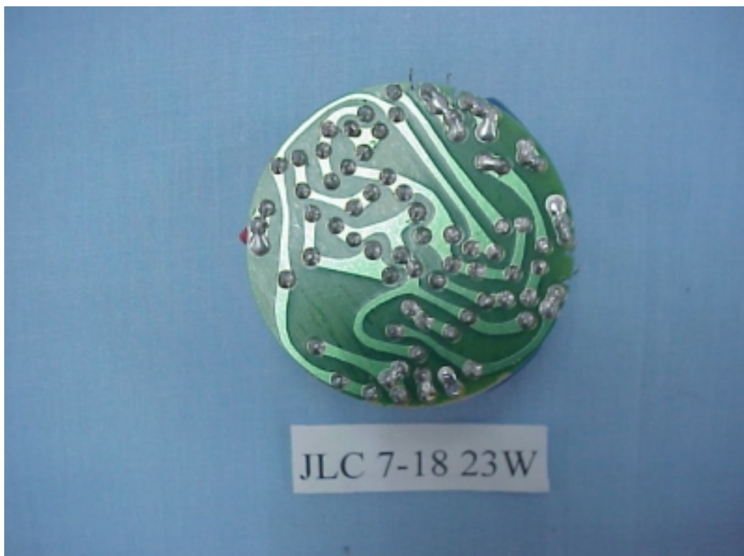
Figure 9 ENERGY SAVING LAMP (M/N: JLC 7-18 23W) MAIN BOARD (SOLDERED SIDE)
