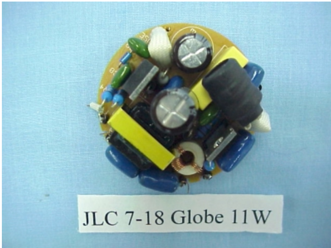
Figure 2 ENERGY SAVING LAMP (M/N: JLC 7-18 GLOBE 11W) MAIN BOARD (COMPONENT SIDE)
