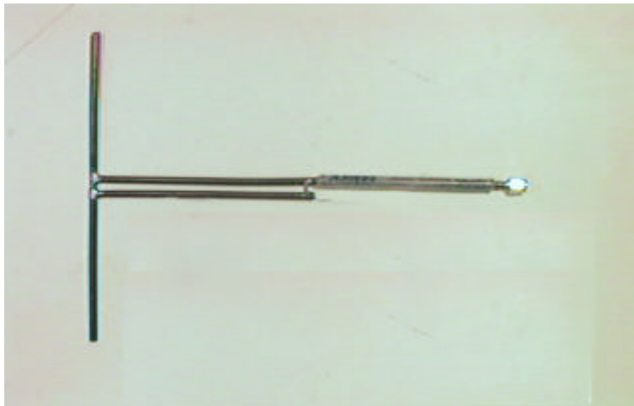
Reference Dipole Antenna Used for ERP Measurement
