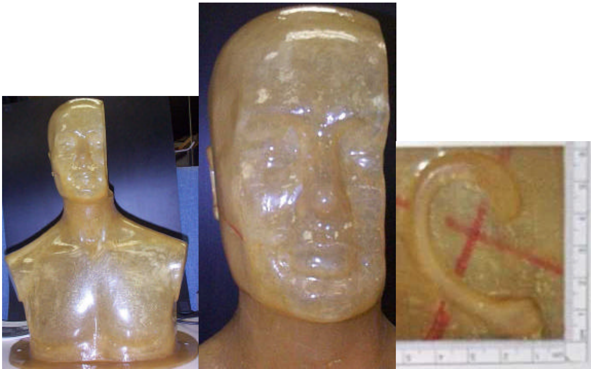
Figure 5. Right hand “realistic” phantom used for verification measurements.
