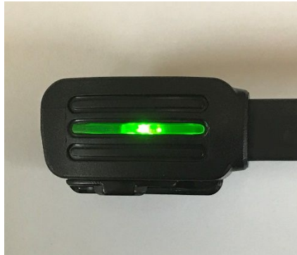
Solid green LED indicates successful in-fleet
