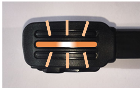
Figure 15 Start with Slow Orange LED, Ready to Train Physical Fobs
