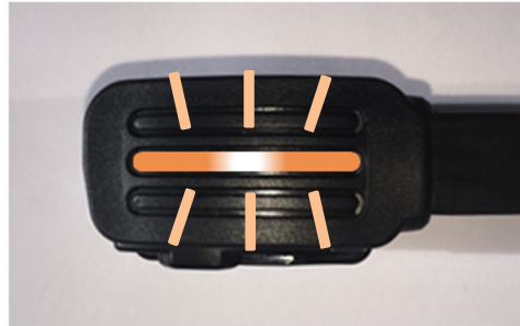
Figure 19 Start with Slow Orange LED, Ready to Train 2nd Physical Fob
