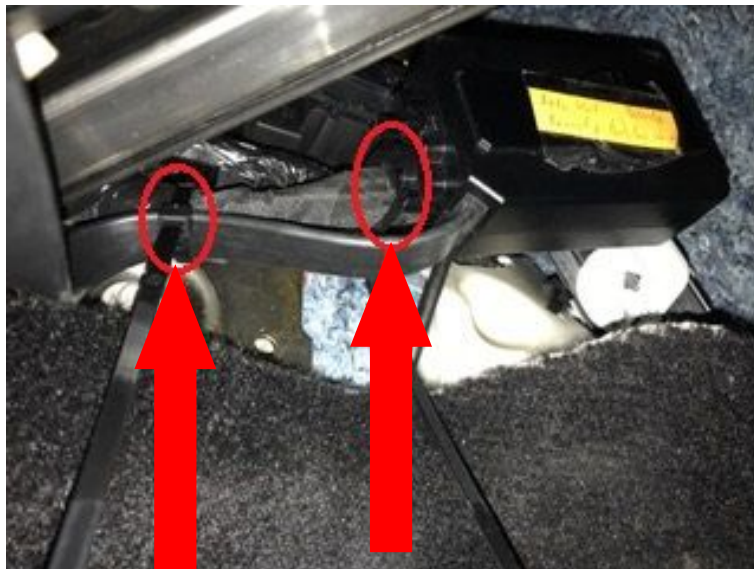
UTP 1.0 securely tie wrapped onto wire harness. In this example, one side of the UTP 1.0 is tie wrapped and UTP cable is tie wrapped onto the wire harness as well.
