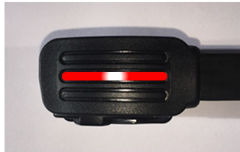
Figure 10 Solid Red LED Indicates Failed In-Fleet
