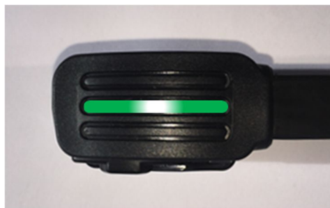
Figure 20 Solid Green LED, Fob Training Complete
