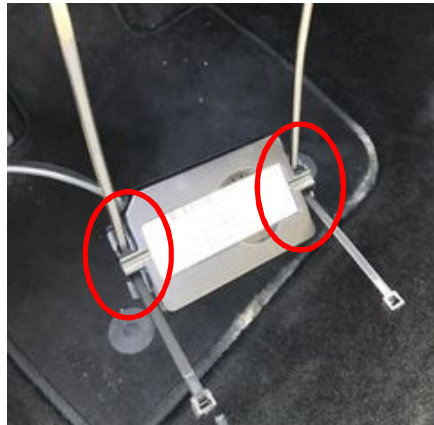
Tie wraps fed through inserts on both ends of UTP 1.0
