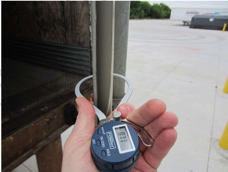
Measure overall door thickness with external caliper
