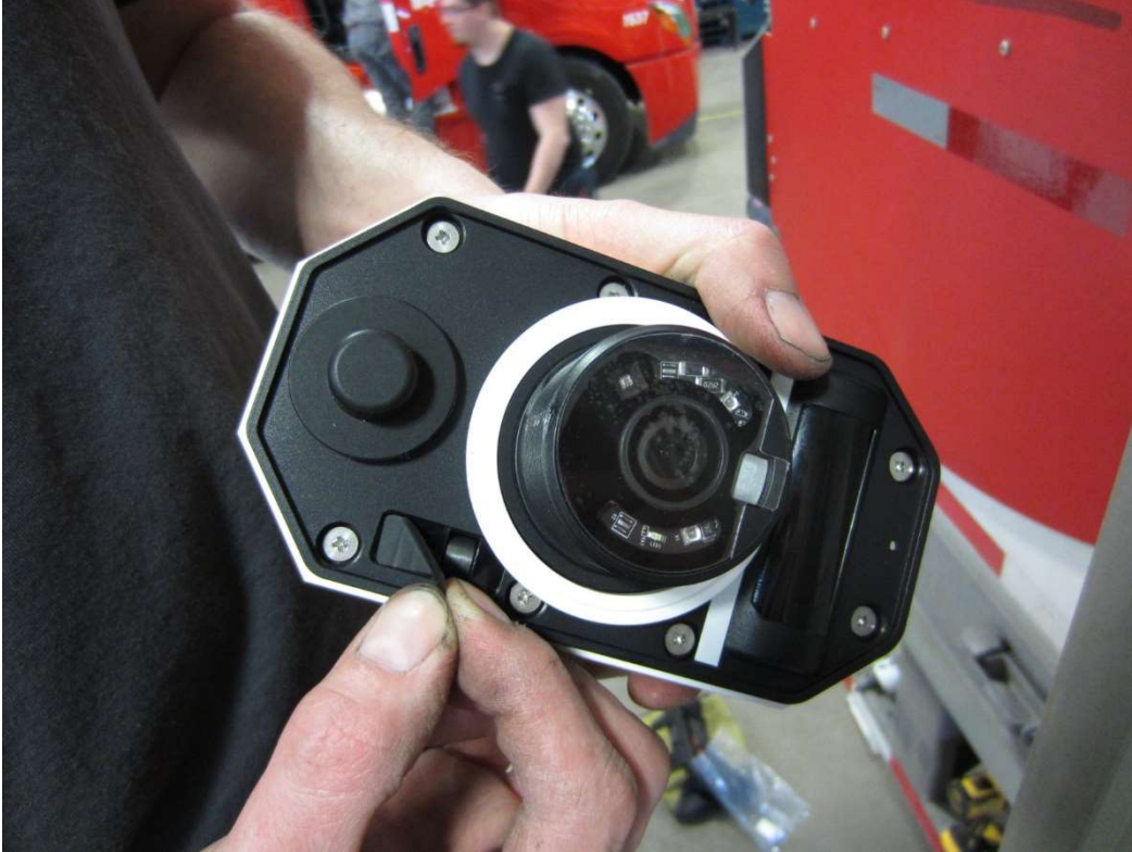
Removing tape over activation magnet
