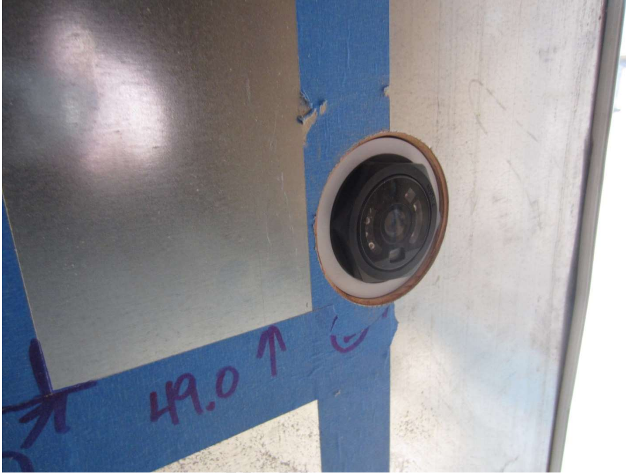
Interior washer and nut installed in countersink
