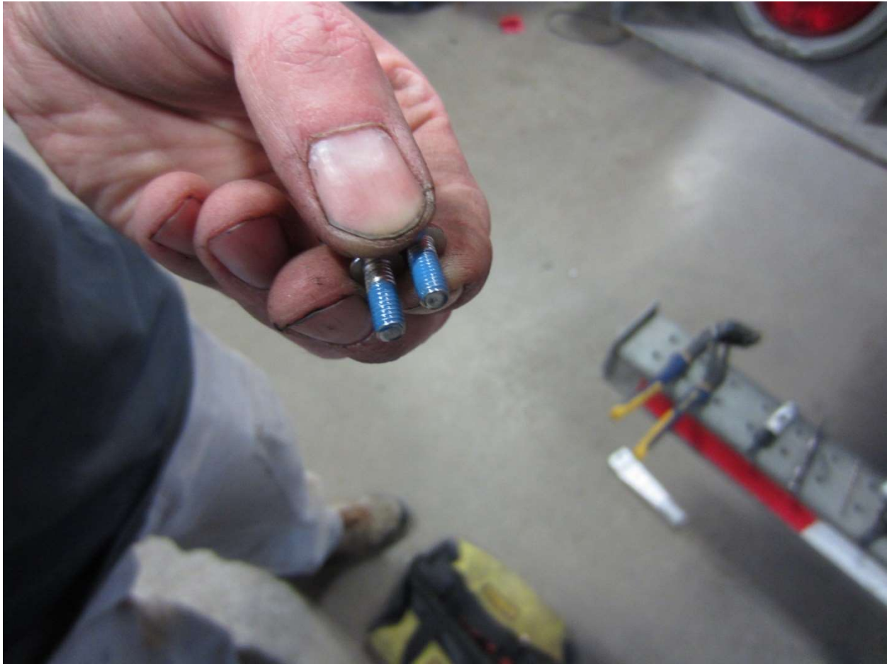
Loctite applied to thread forming screws
