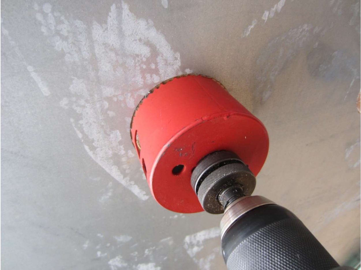
Drill 3 3/8" hole through interior door sheathing
