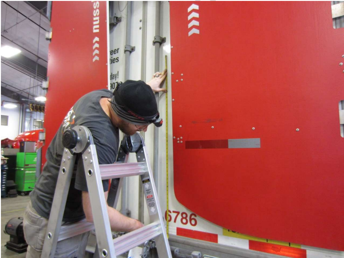
Measure and mark location 50" up from trailer floor
