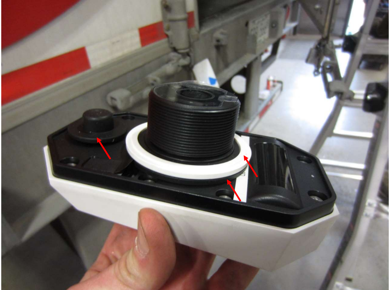
External shock mount hardware
