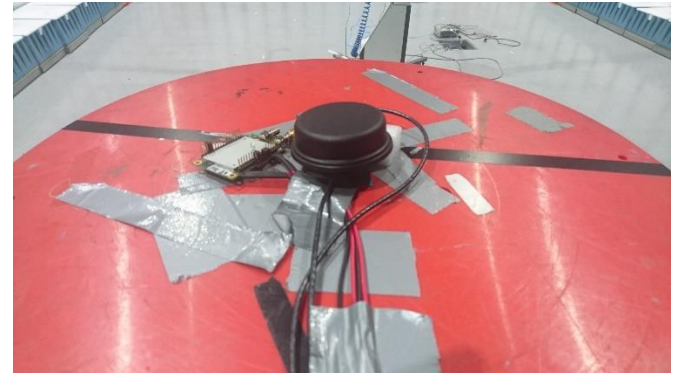
Radiated emissions above 1 GHz with monopole antenna
