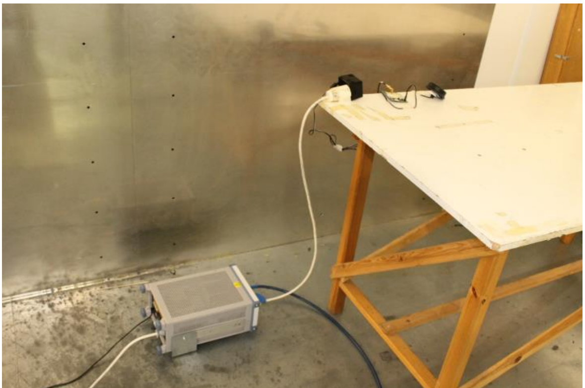
Photograph 2. AC power line conducted emissions test setup (setup4)
