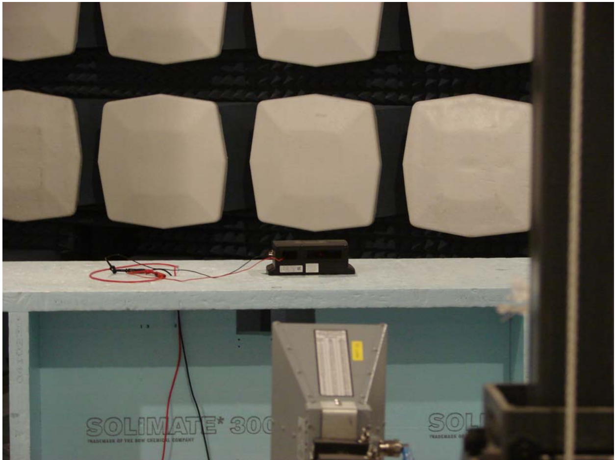
Picture 2: Receiver Radiated emission test setup 1 GHz – 5 GHz
