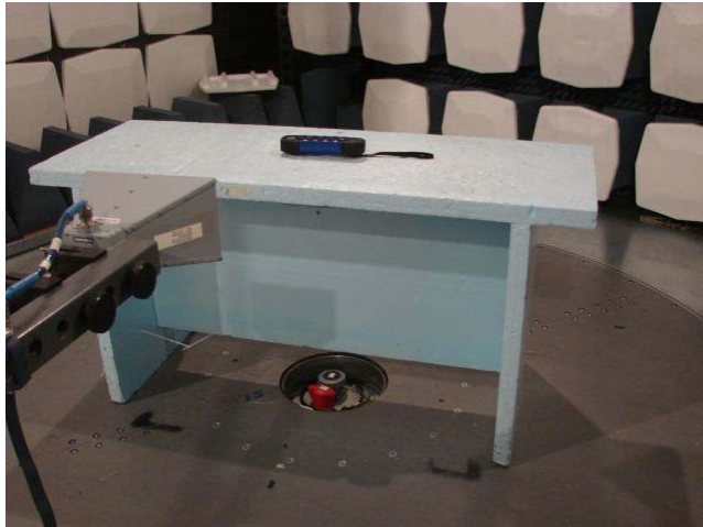
Picture 3: Transmitter Radiated emission test setup 1 GHz – 10 GHz.
