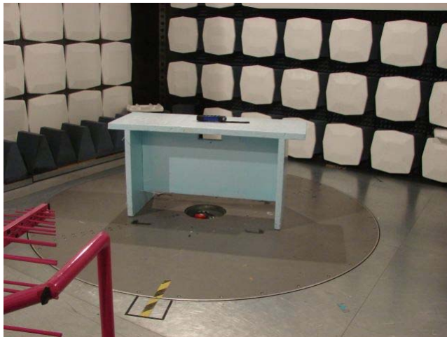
Picture 2: Transmitter Radiated emission test setup <1 GHz
