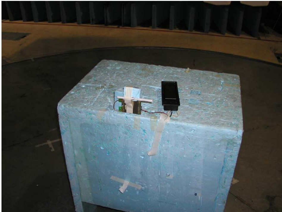
Photograph 6 Radiated emissions test setup
