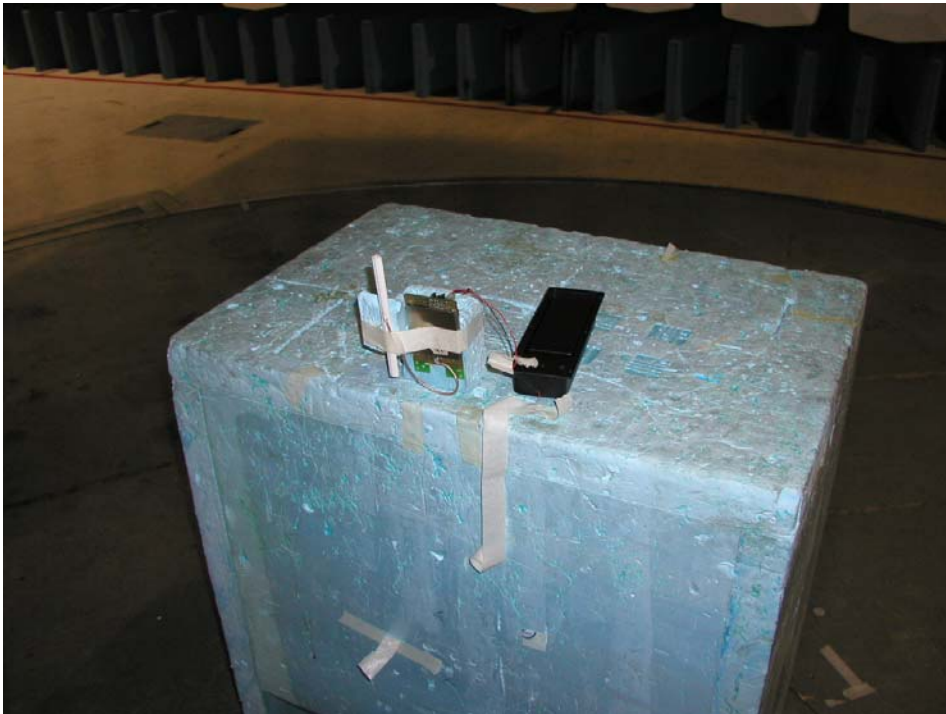
Photograph 4 Radiated emissions test setup
