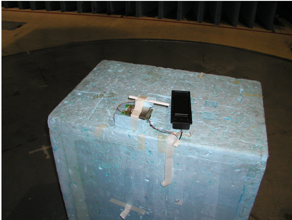
Photograph 5 Radiated emissions test setup
