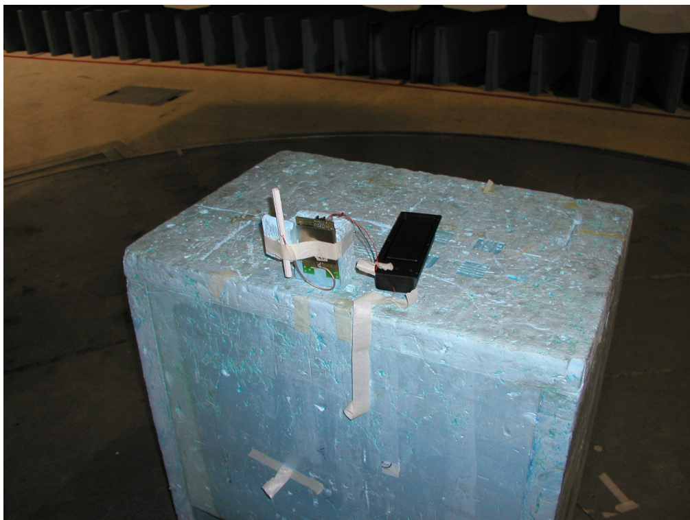
Photograph 4 Radiated emissions test setup
