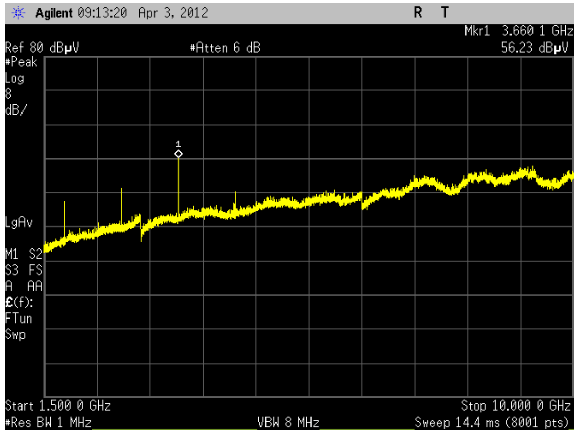
Figure 26. Radiated spurious emissions, middle channel
