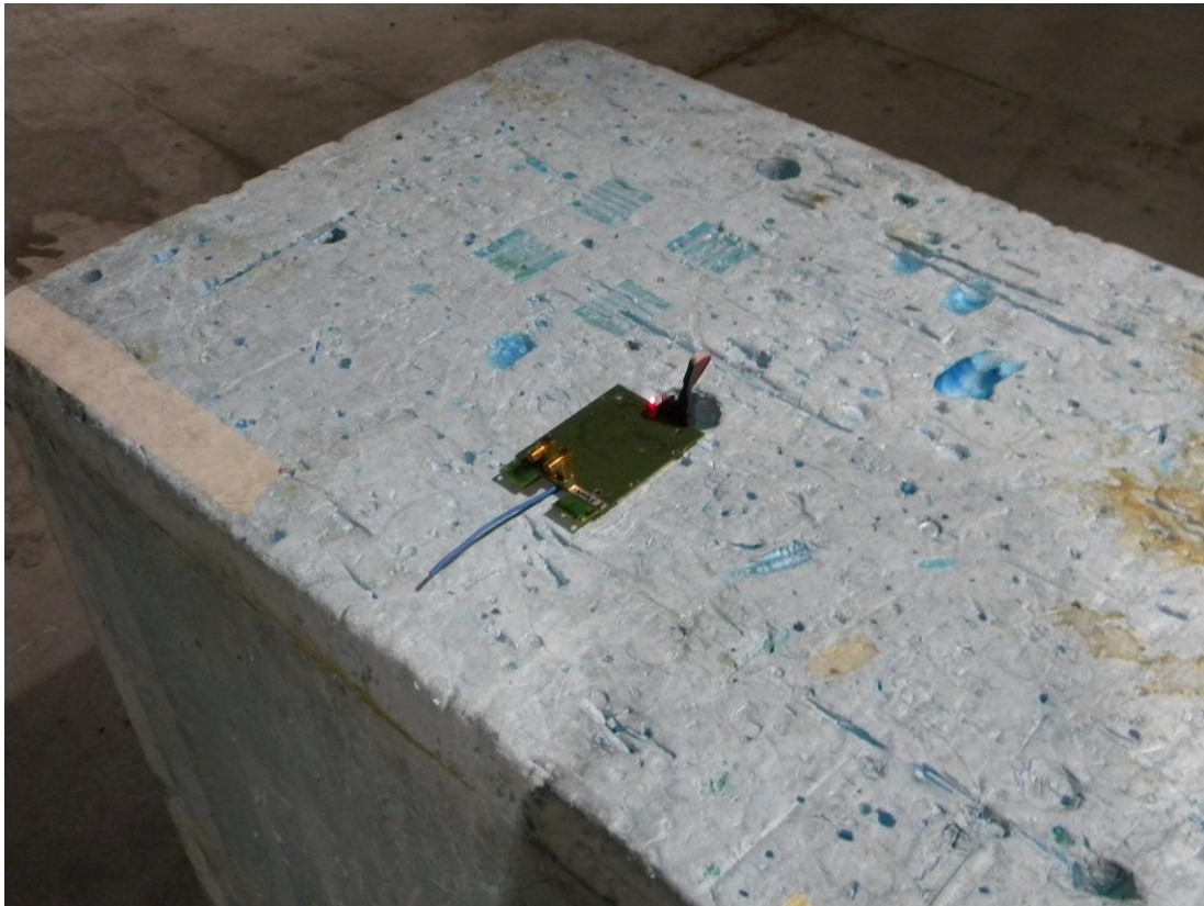
Photograph 1. Radiated emissions test setup, antenna 1.
