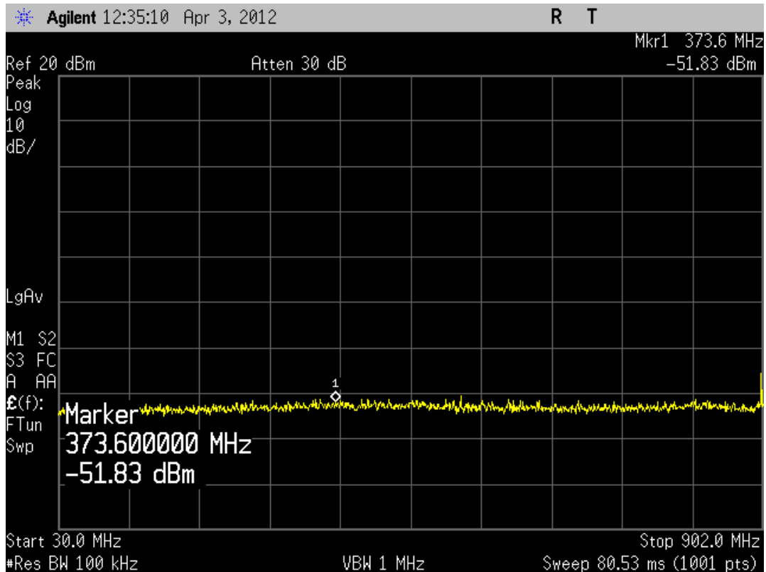
Figure 20. Conducted spurious emissions, middle channel
